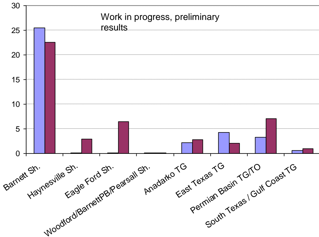
Figure 11. Estimated hydraulic fracturing water use in 2008 and 2010 in the state of Texas.
