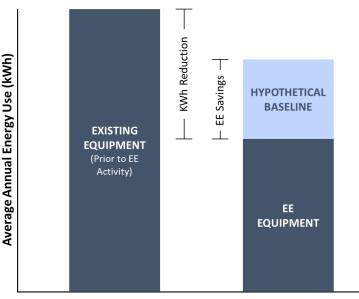
Comparison of Total kWh Reduction vs. EE Savings Using a Hypothetical Baseline for the Installation of New Equipment
