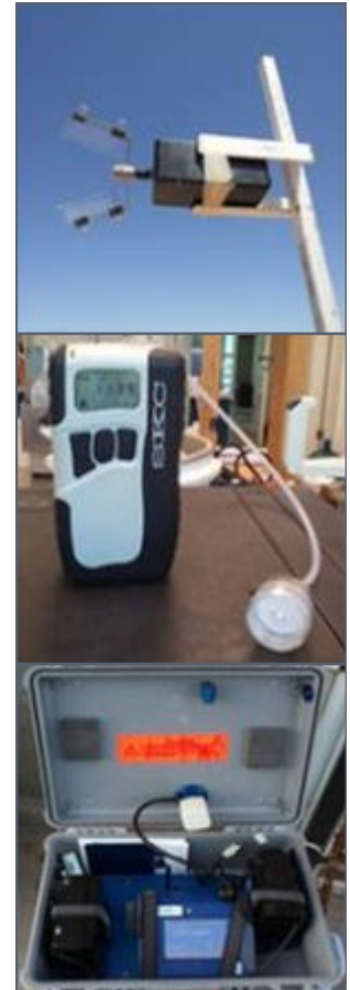
Instruments used to measure PM from dust storms, and for experiments in unpaved roads.
