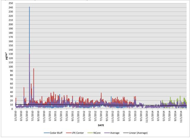
Figure 11. 24-hr Avg. PM<sub>2.5</sub> Continuous Monitoring Data w/ Trendline 2010-2014
