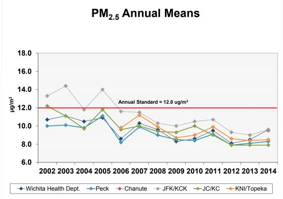
Figure 12. Annual Avg. Filter Based PM<sub>2.5</sub> Monitoring Data 2002-2014
