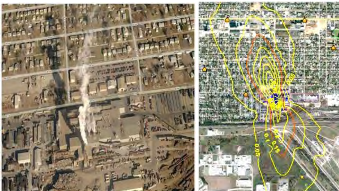
Local Air Pollutant Example. Industrial lead emissions (left) and modeled hotspot (right). The area inside the orange contour is predicted to violate the NAAQS.
