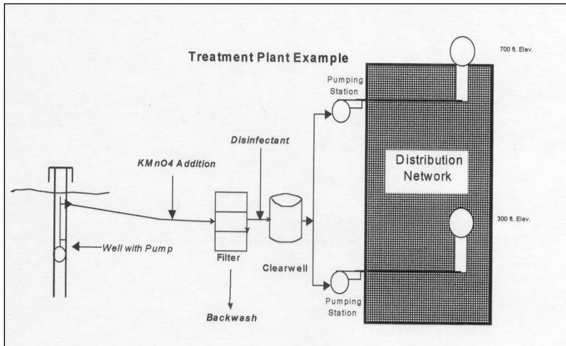
Layout maps are more detailed than schematics and contain more specific information on the location and orientation of physical facilities. In collecting the layout data, a surveyor may easily obtain the latitude and longitude data of a PWS by using portable GPS equipment. A water system may have separate layout maps for its treatment plant and distribution system.
