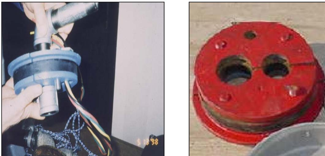
The other type of seal is an overlapping exterior sanitary well seal, illustrated in Exhibit 4.3. It is commonly used in outdoor applications with submersible pumps and pitless adapter units. The vent is under the lip, and gasket material seals all openings around the casing and conduit.
