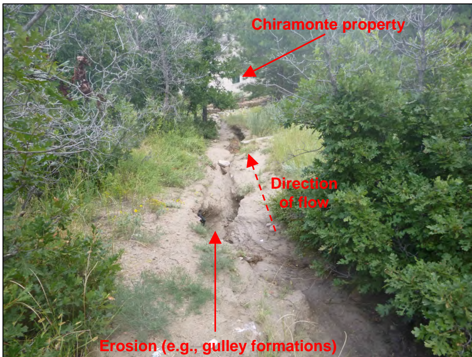
Photograph 62. Additional view of erosion (e.g., gully formations) on private property located downgradient of the MS4 outfall pipe. Note the location of the Chiramonte private property and residence located directly downstream of this drainage area.
