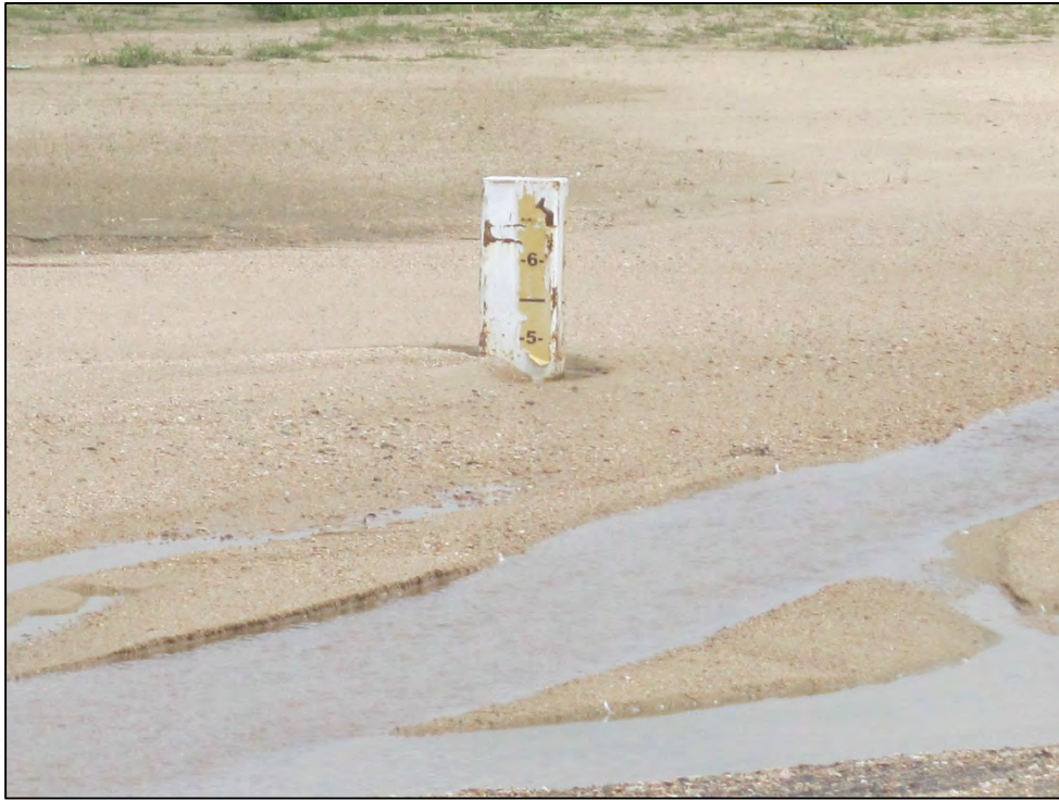
Photograph 115. Additional view of one of six fixed vertical sediment markers with a reading of approximately five feet.
