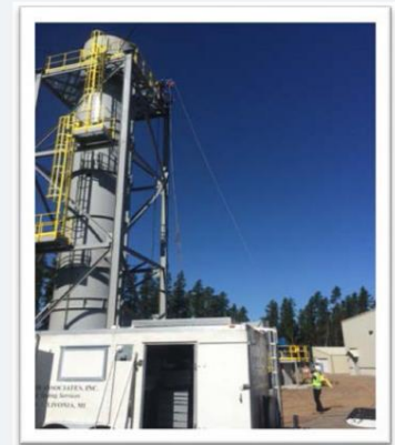
The CEMP deployed the portable air monitoring equipment to collect ambient air quality data at the Mine Ventilation Air Raise (MVAR) during the Michigan DEQ required stack test on September 16.
