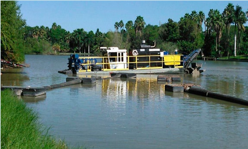
Floating dredger from IMS Dredges® is self-propelled and has a 9-foot cutterhead. Sediment is transported via floating pipe to an offsite dewatering system. Credit: Brownsville Public Utilities Board.
