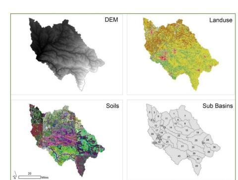
Figure 4. An example of SWAT mode inputs: digital elevation, land use, soils, and sub-basin maps.
