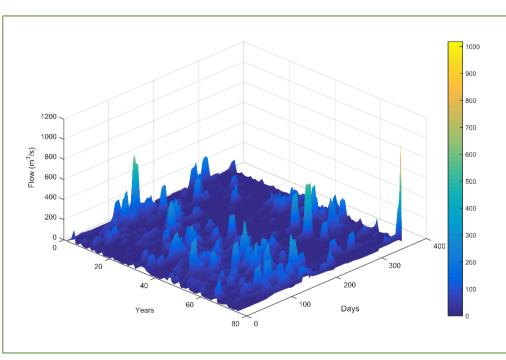
Figure 3. Daily cubic meters of water discharge in Spring River. By running different land-use scenarios in SWAT we can test how stream discharge can change over time.
