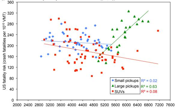
Figure 4.12. US fatality risk per VMT vs. curb weight, light truck models
