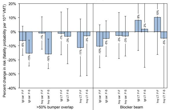
Figure 6.11. Effect of compatibility measures on risk imposed by light trucks on other lightduty vehicles, by crash partner vehicle type and crash configuration
