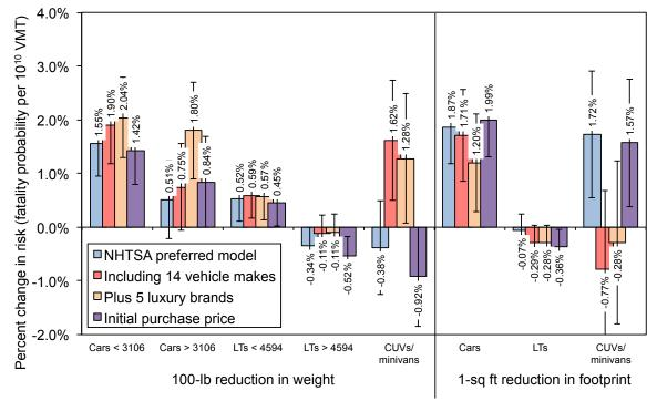
Figure 5.3. Estimated effect of mass or footprint reduction on US fatalities per VMT, after controlling for vehicle manufacturer or for initial vehicle purchase price, by vehicle type
