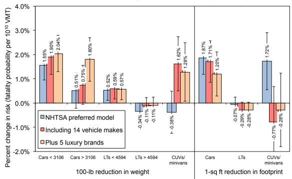
Figure 5.2. Estimated effect of mass or footprint reduction on US fatalities per VMT, after controlling for vehicle manufacturer, by vehicle type
