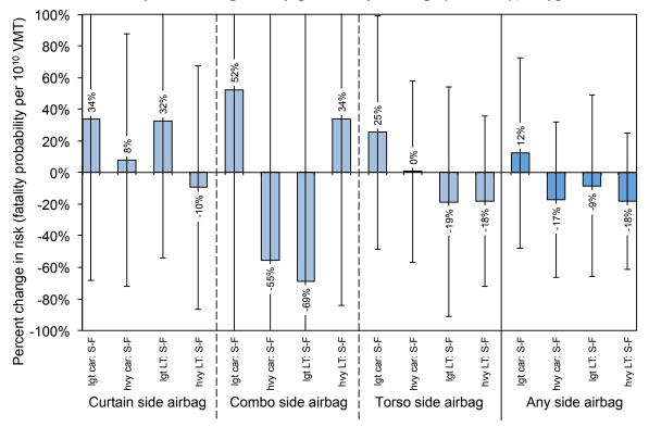
Figure 6.6. Estimated effect of side airbags on risk to <u>light truck occupants only</u>, when struck in the side by another light-duty vehicle, by crash partner vehicle type
