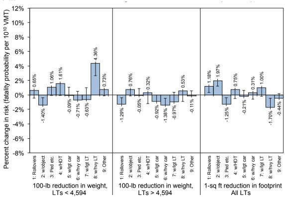
Figure 2.3. Estimated effect of mass or footprint reduction on risk in light trucks, by type of crash
