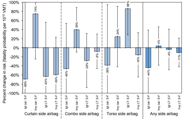
Figure 6.5. Estimated effect of side airbags on risk to <u>CUV/minivan occupants only</u>, when struck in the side by another light-duty vehicle, by crash partner vehicle type
