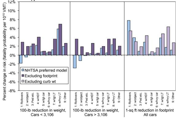
Figure 3.4. Estimated effect of reduction in car mass or footprint on US fatality risk per VMT, by crash type
