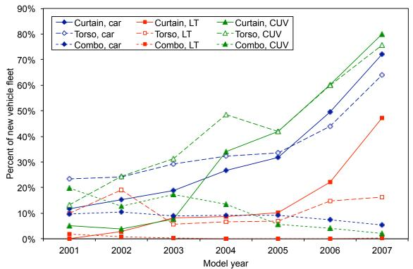
Figure 6.3. Market penetration of side impact airbags, by vehicle type and model year
