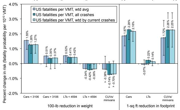
Figure 2.1. Estimated effect of mass or footprint reduction on US fatality risk per VMT, across all crash types and weighted average effect in each type of crash, by vehicle type
