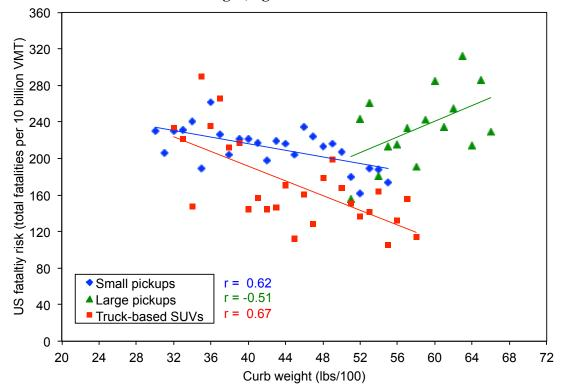
Figure 4.3. Relationship between US fatality risk and curb weight, with vehicles grouped into 100-lb increments of curb weight, light trucks
