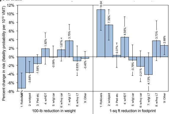
Figure 2.4. Estimated effect of mass or footprint reduction on risk in CUVs/minivans, by type of crash
