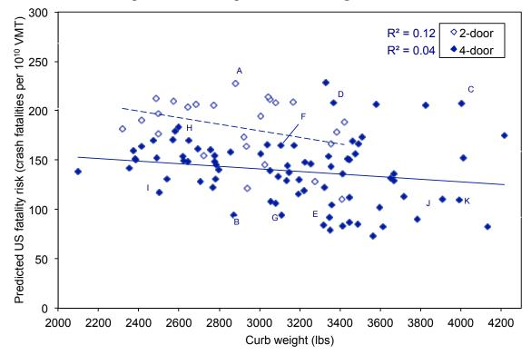
Figure 4.10. Predicted US fatality risk per VMT after accounting for all driver, crash, and vehicle variables except mass and footprint vs. curb weight, car models
