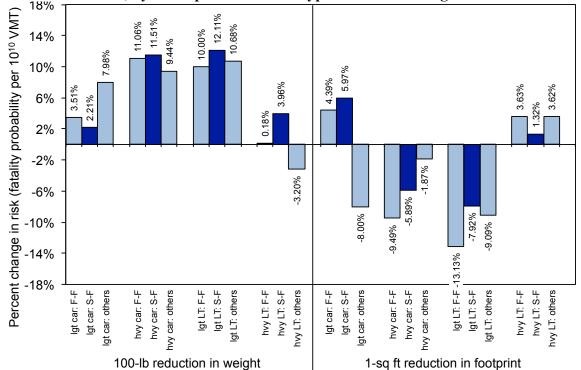
Figure 6.8. Estimated effect of mass reduction on risk to <u>CUV/minivan occupants only</u> in two-vehicle crashes, by crash partner vehicle type and crash configuration
