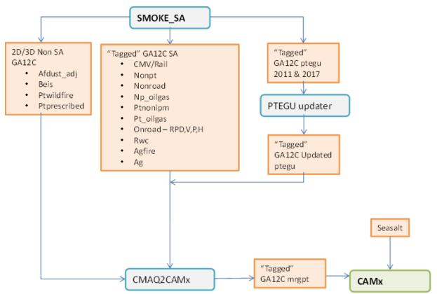
Figure 12. SMOKE processing procedures for CAMx-APCA modeling.
