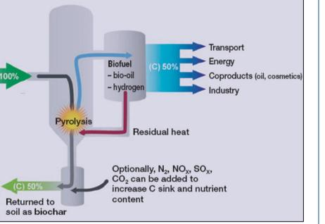
**Figure 3: Biochar from Pyrolysis**
