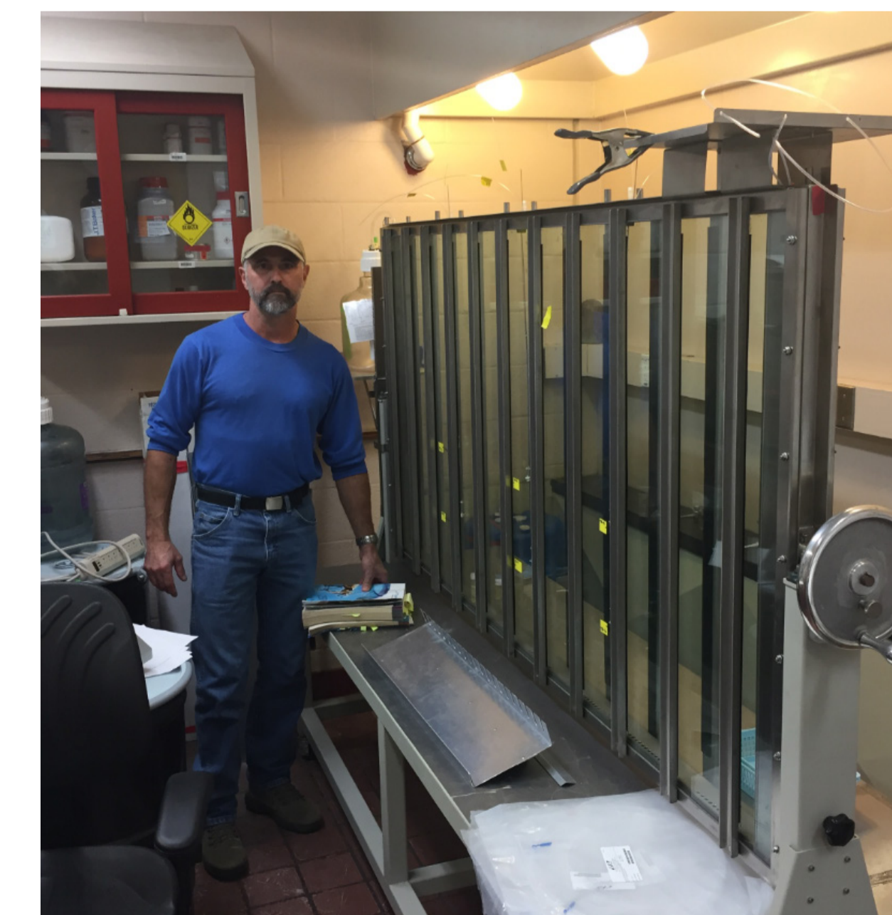
Figure 5. A sand tank is being prepared to generate model test data.
