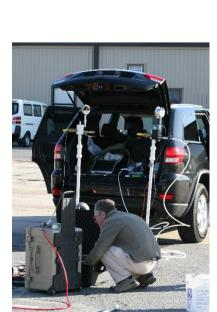
Pneumatic slug tests
