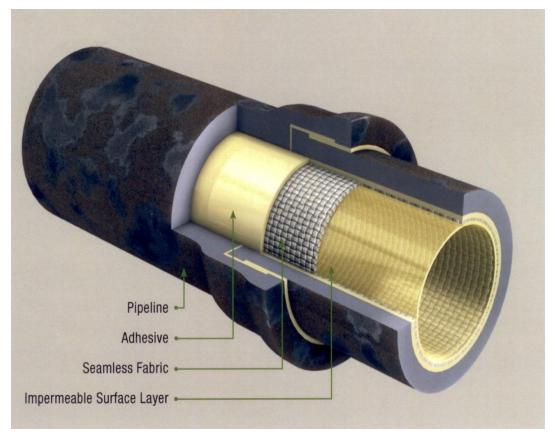
The liner is a seamless/joint-less circular woven fabric-hose made of polyester yarns and a plastic coating (PU/PE) which is bonded as inner liner into the host pipe using a solvent-free two-component adhesive.
