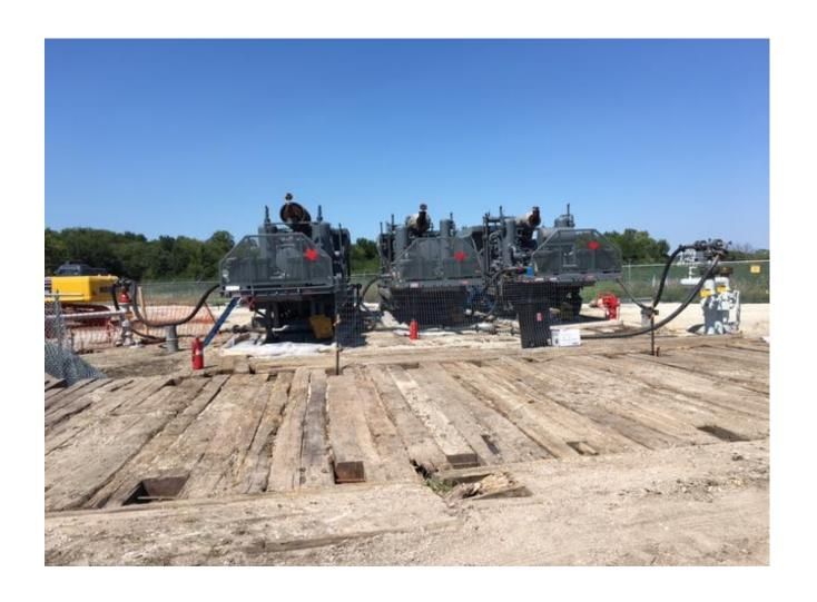
Three 300-hp compressors in parallel operation
