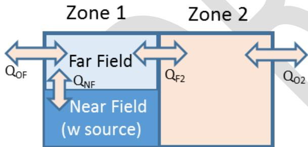
Figure 2. Air Flows in the Near-Field Far-Field Model
