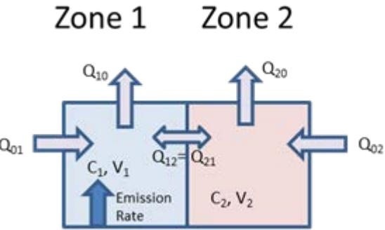
**Figure 1: Schematic of two zone model of indoor environment**
