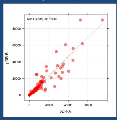
Comparison of BC concentrations (µg/m³) measured using two different microAethalometer units
