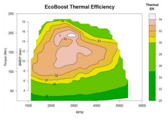
Figure 6. EcoBoost® Thermal Efficiency
