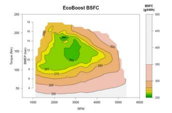
Figure 5. EcoBoost® BSFC (g/kWh)
