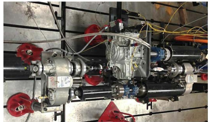
Figure 5. GM6T40 Transmission during testing
