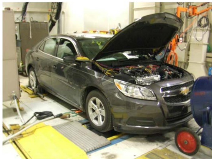
Figure 1. Chevy Malibu undergoing dynamometer testing
