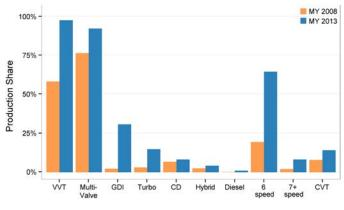
Figure 5. Five year change in light-duty vehicle technology penetration share
