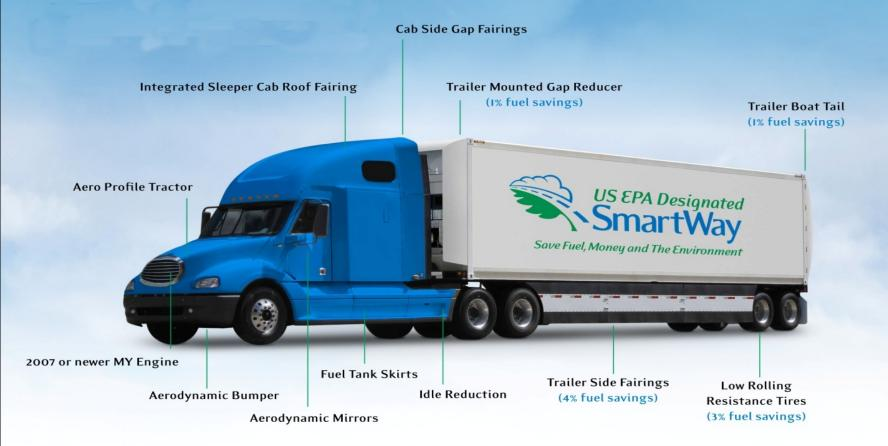
A SmartWay tractor and trailer annually save 2,000 to 4,000 gallons of fuel and reduce CO2 emissions by up to 20% as compared to similar trucks on the road. Learn more at www.epa.gov/smartway
