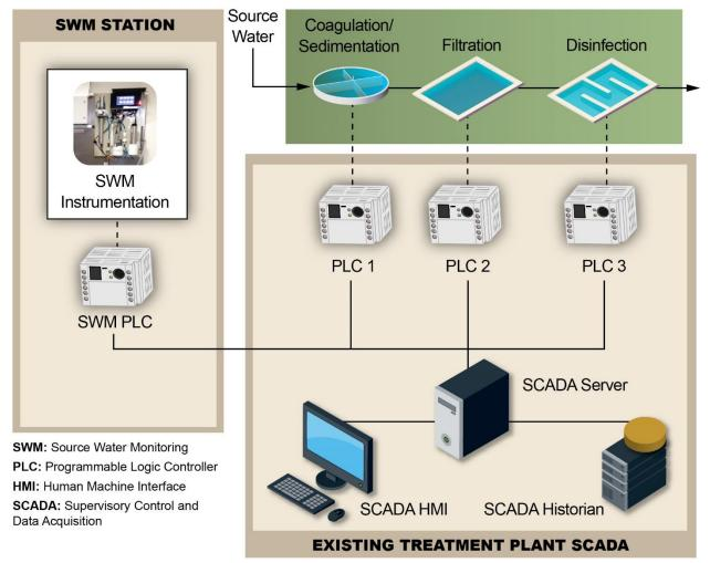
Figure 6-7. SWM Information Management as an Extension of an Existing SCADA Architecture
