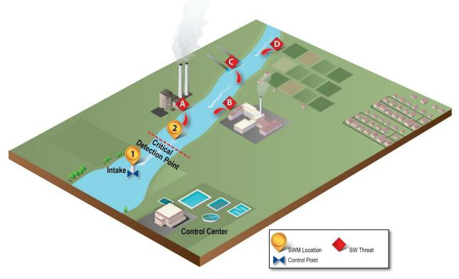
Figure 3-2. A Single Upstream SWM Location to Monitor Multiple SW Threats
