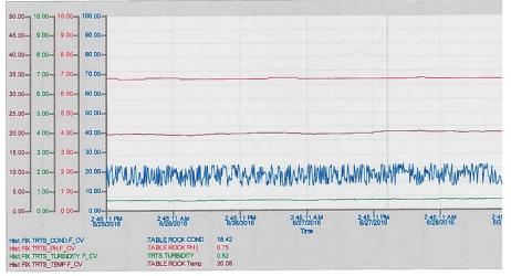
Figure 9-2. Example of Greenville Water SCADA System Screen for SWM Data
