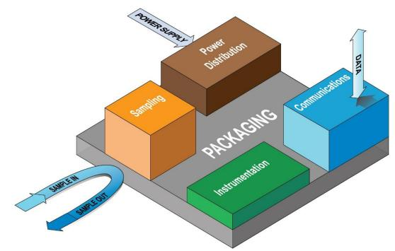
Figure 5-1. Functional Block Diagram of an SWM Station
