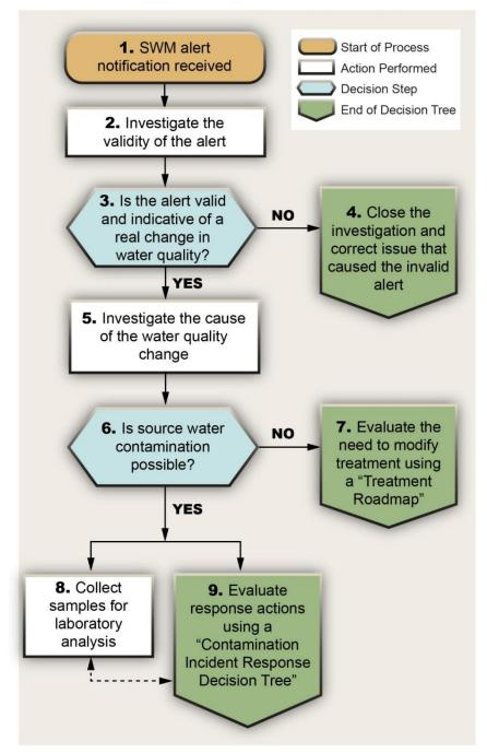
Figure 7-1. Example of an SWM Alert Investigation Process Flow Diagram
