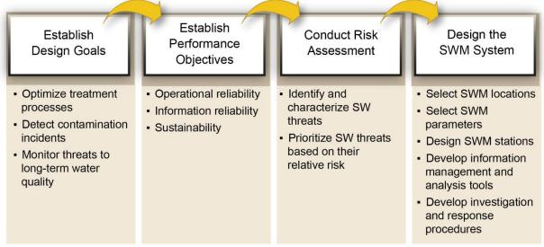
Figure 2-1. Source Water Monitoring Implementation Framework
