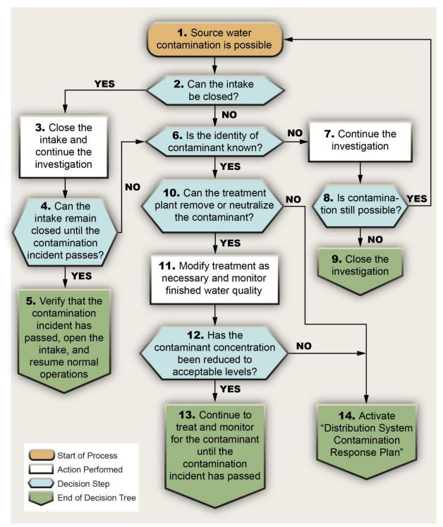
Figure 7-3. Example Source Water Contamination Incident Response Decision Tree
