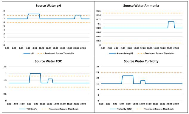
Note that this figure displays idealized data, without noise, to clearly demonstrate the concept of threshold analysis. Figure 6-1. Time-Series Plots and Thresholds for Treatment Process Optimization
