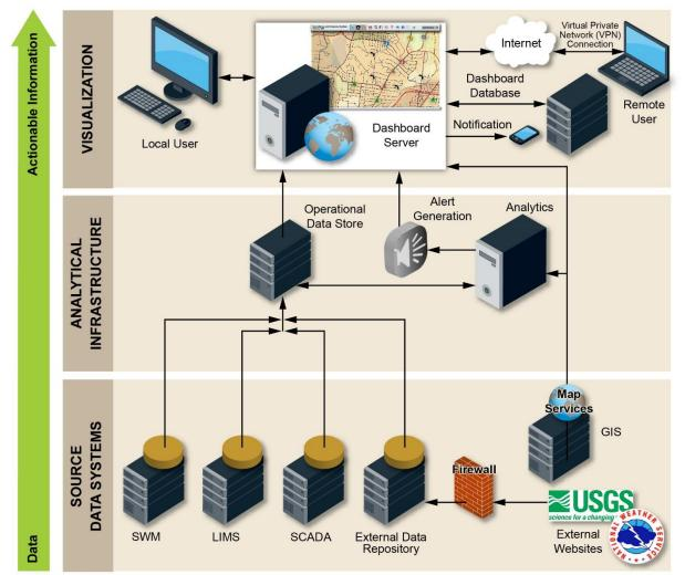
SWM: Source Water Monitoring LIMS: Laboratory Information Management System SCADA: Supervisory Control and Data Acquisition
