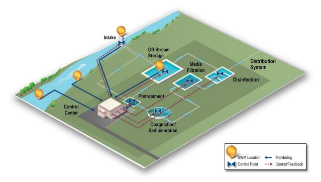
Figure 1-2. Example Schematic of Source Water Monitoring
