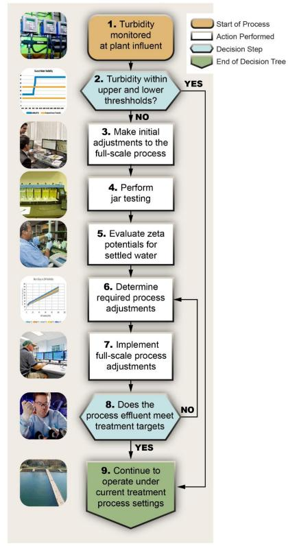
Figure 7-2. Example Treatment Optimization Procedure Flow Diagram
