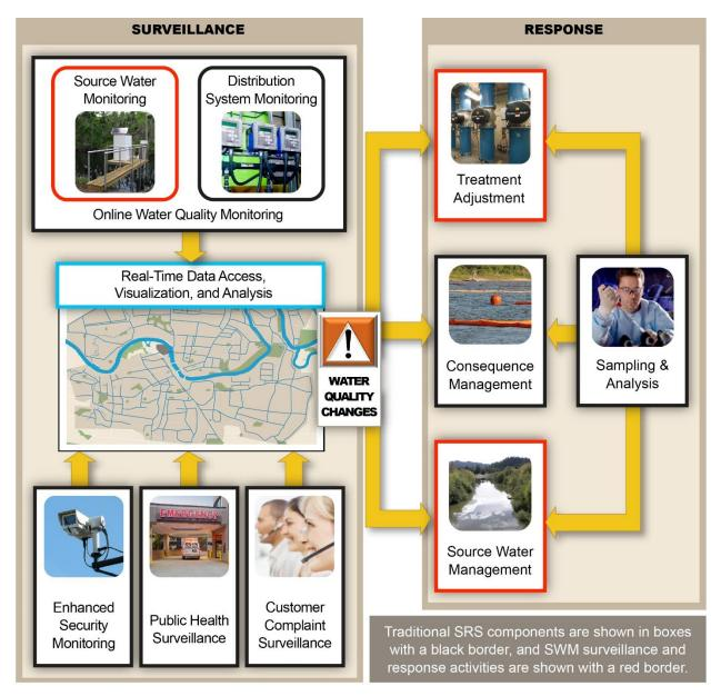
Figure 1-1. Incorporation of Source Water Monitoring into an SRS
