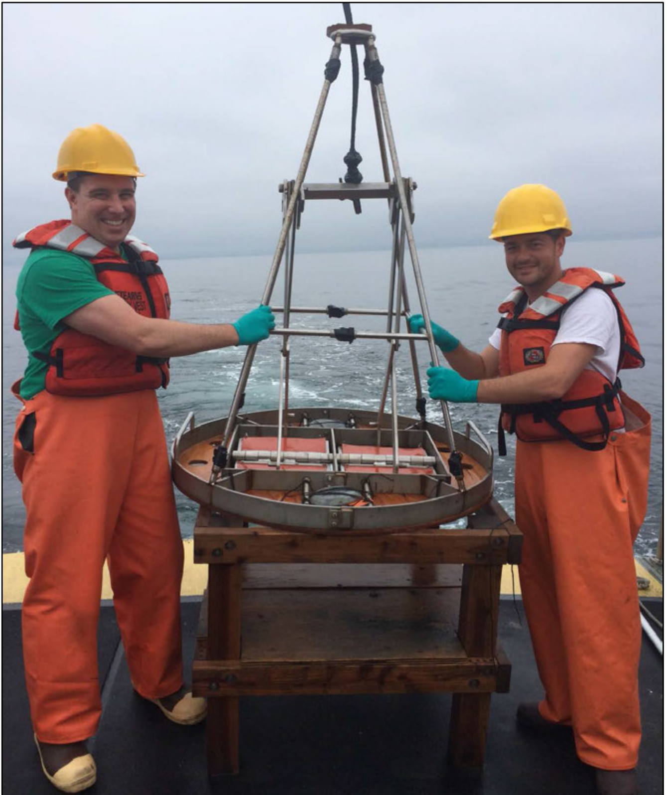
Figure 23. Double Van Veen sediment grab sampler being deployed from the Coral Sea.
