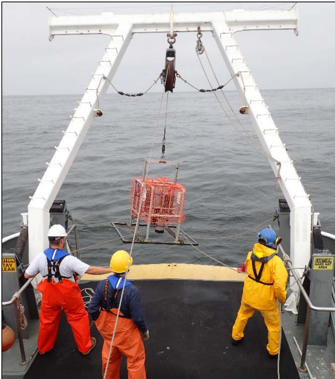
Figure 12. SPI/PVP camera system being deployed from the Coral Sea in 2014.
