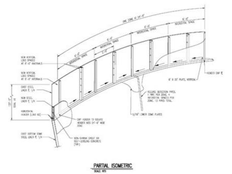
angles welded to the existing steel line at 3'-0" on center
