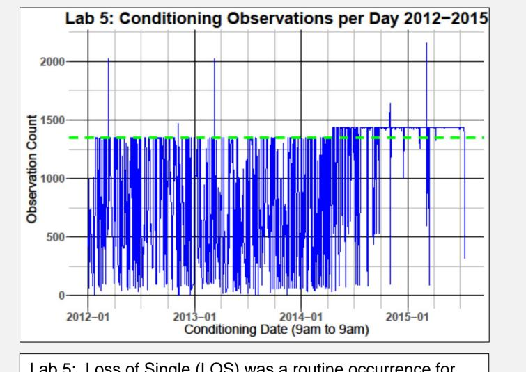
Lab 5: Loss of Single (LOS) was a routine occurrence for the data logger recording the environmental conditions. Mean RH and Temp. were not based on a complete 24-hr period until late 2014.
