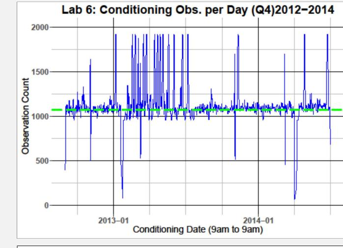
Lab 6: Good and complete logging of data. Observing "double counting" of minute readings is not uncommon. Only infrequent Loss of Single (LOS).
