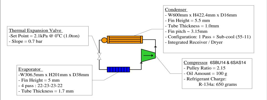
All components were common during testing of the 6SBU14 and 6SAS14 compressors.
