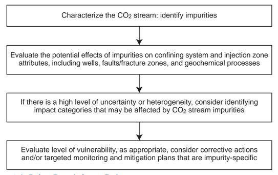
Figure 3.4. Carbon Dioxide Stream Evaluation
