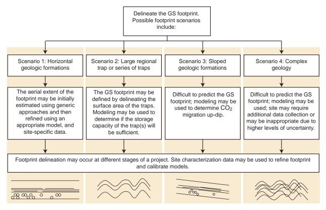
Figure 3.5. Geologic Sequestration (GS) Footprint Delineation
