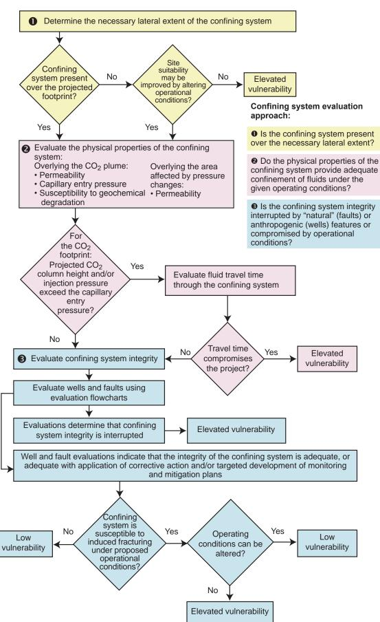
Figure 3.2. Confining System Evaluation
