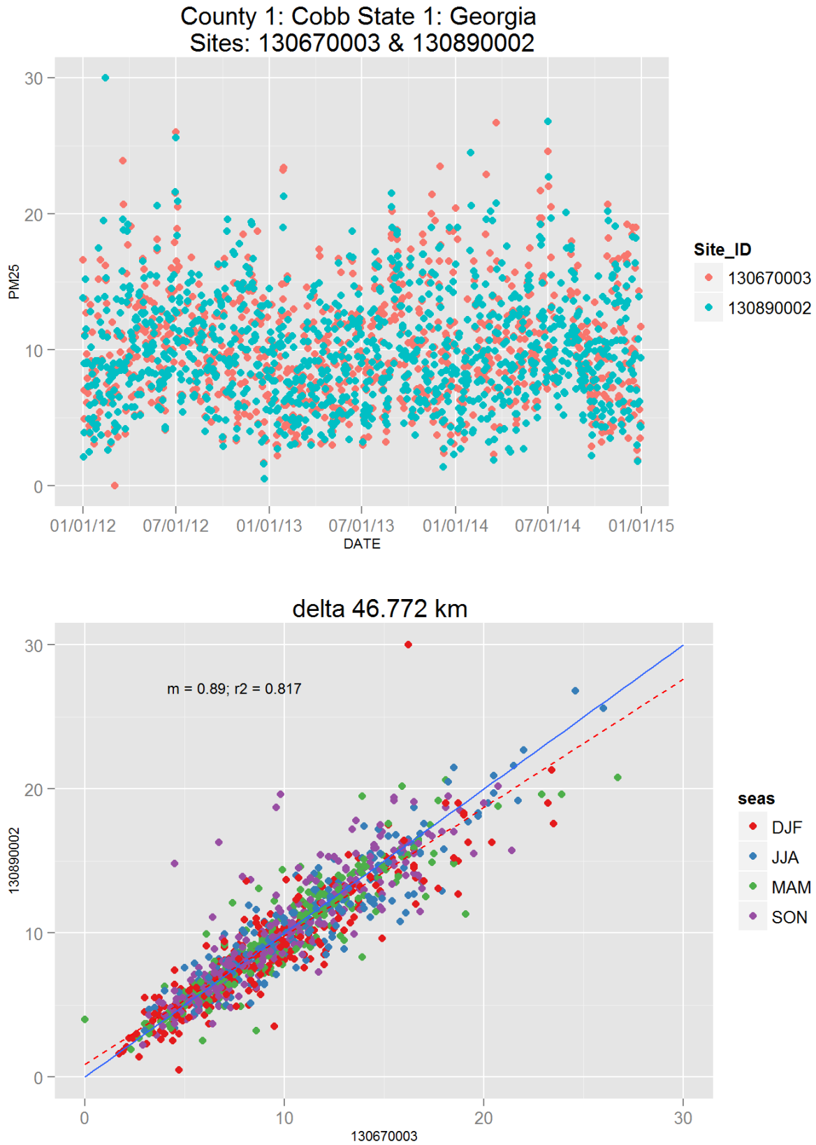
Figure 93: Comparison of PM 2.5 data for sites 130670003 and 130670003. Top panel shows time series for both sites for years 2012-2014. Bottom panel shows scatter plot of paired data, along with slope for the linear regression and correlation coefficient (r 2 ), with data points are colored by month.
