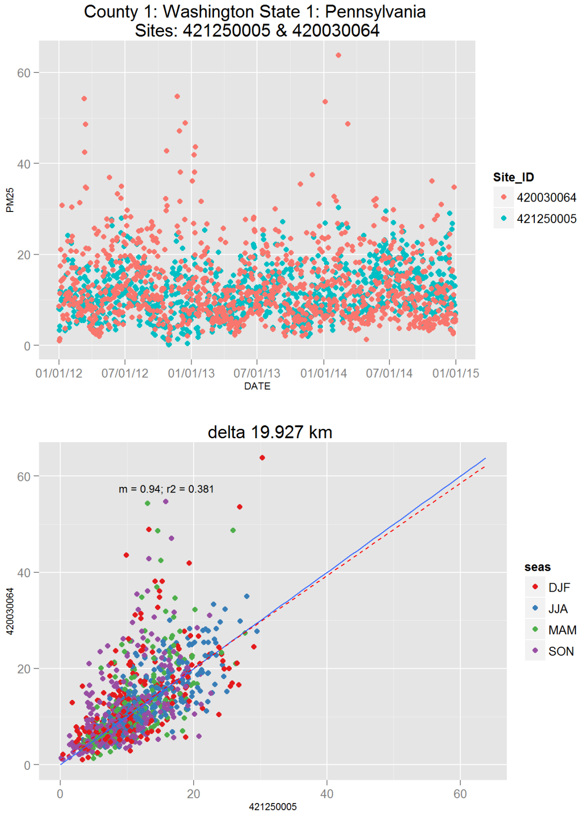
Figure 142: Comparison of PM 2.5 data for sites 421250005 and 421250005. Top panel shows time series for both sites for years 2012-2014. Bottom panel shows scatter plot of paired data, along with slope for the linear regression and correlation coefficient (r2), with data points are colored by month.
