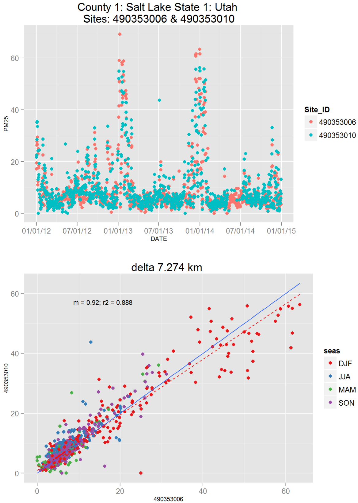
Figure 90: Comparison of PM 2.5 data for sites 490353006 and 490353006. Top panel shows time series for both sites for years 2012-2014. Bottom panel shows scatter plot of paired data, along with slope for the linear regression and correlation coefficient (r 2 ), with data points are colored by month.
