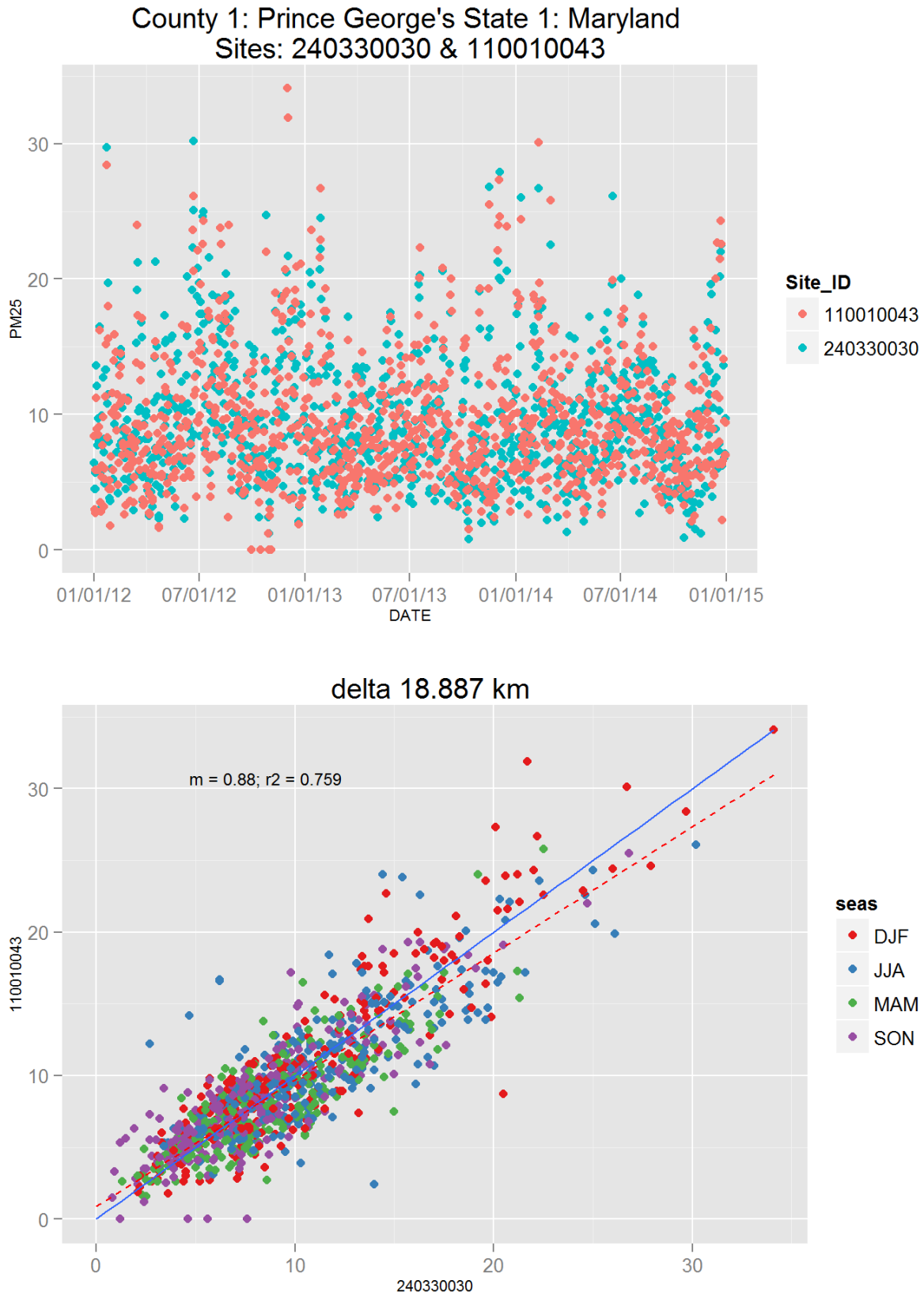
Figure 110: Comparison of PM 2.5 data for sites 240330030 and 240330030. Top panel shows time series for both sites for years 2012-2014. Bottom panel shows scatter plot of paired data, along with slope for the linear regression and correlation coefficient (r 2 ), with data points are colored by month.
