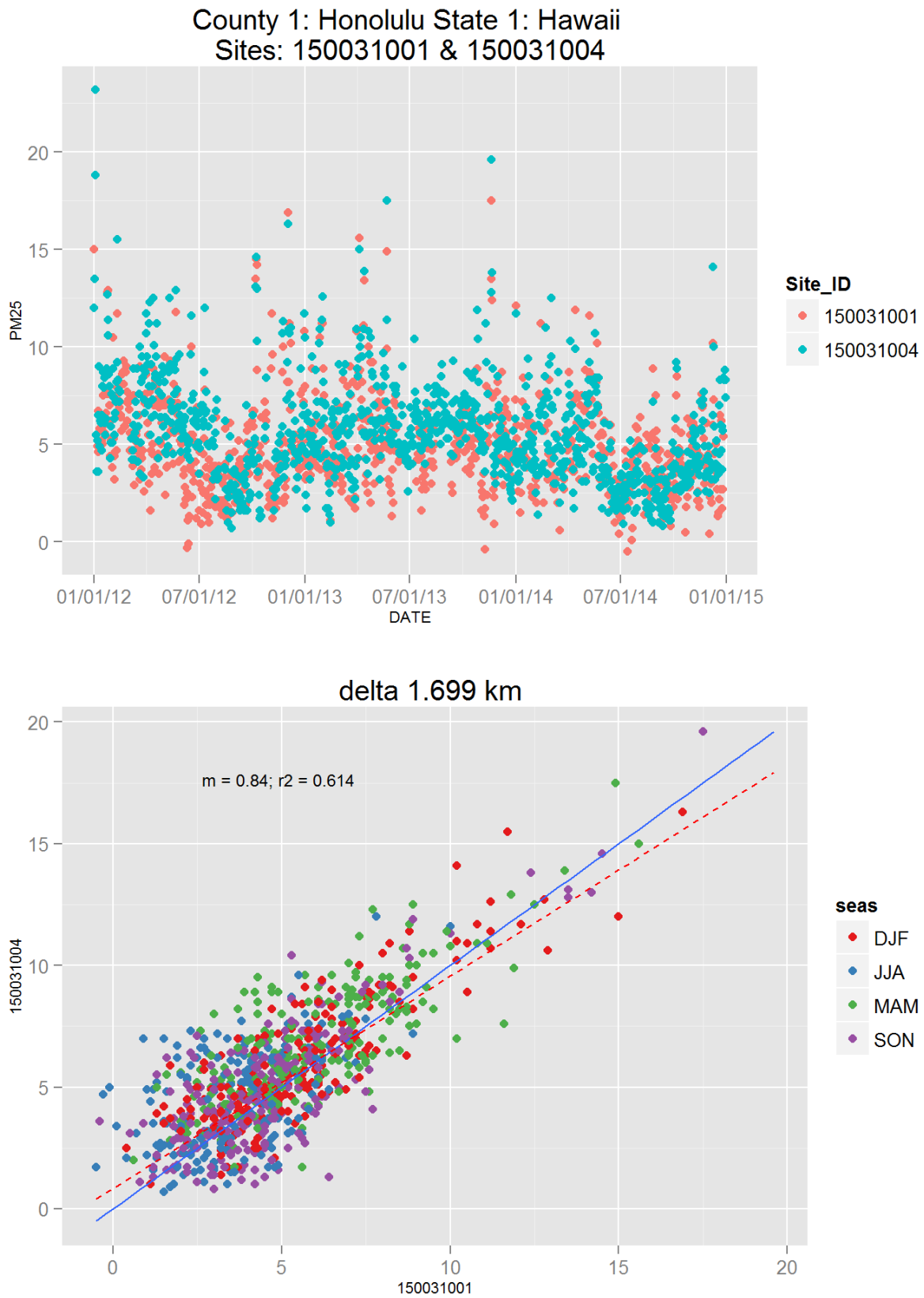
Figure 78: Comparison of PM 2.5 data for sites 150031001 and 150031004. Top panel shows time series for both sites for years 2012-2014. Bottom panel shows scatter plot of paired data, along with slope for the linear regression and correlation coefficient ( r^2 ), with data points are colored by month.
