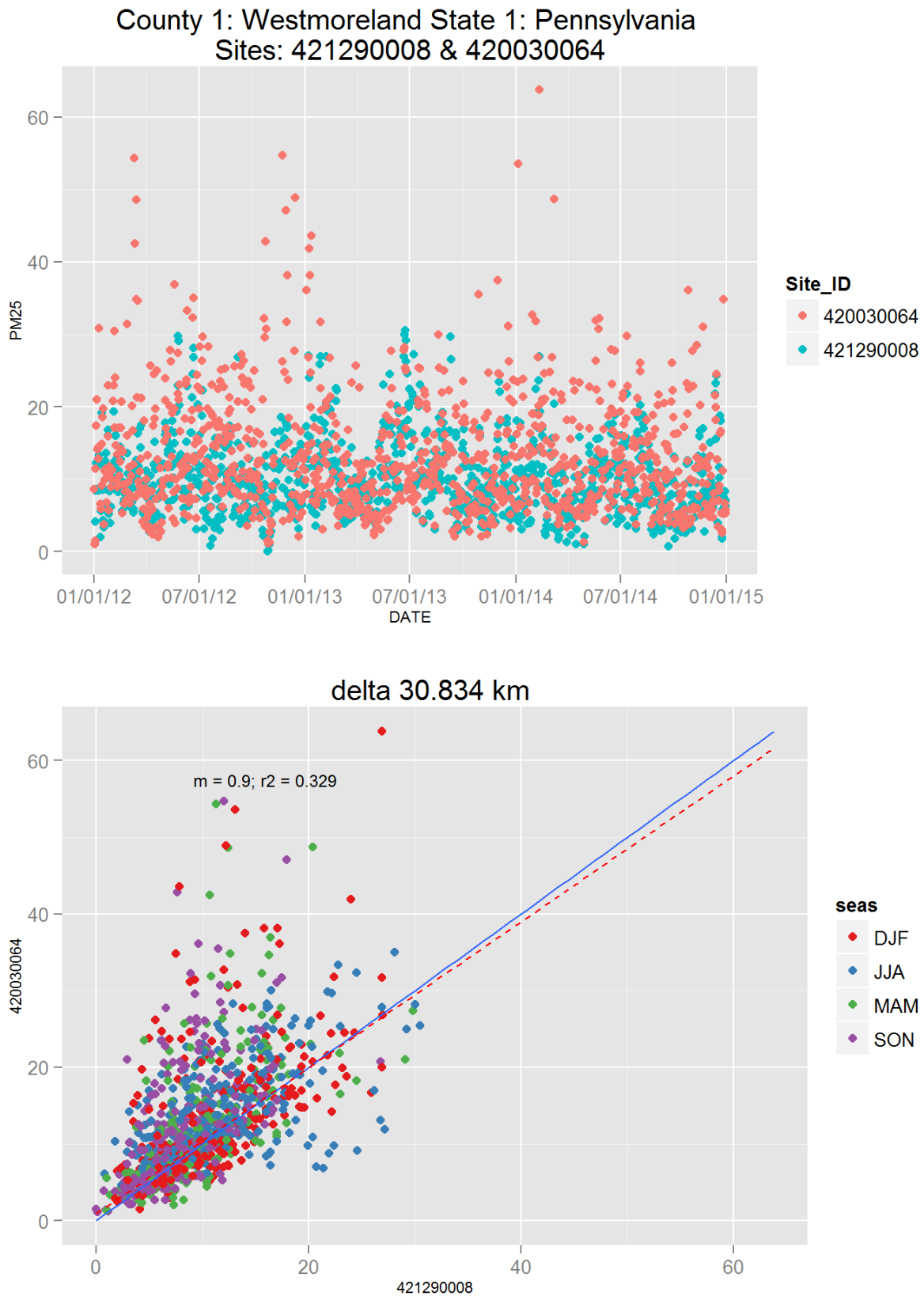
Figure 145: Comparison of PM 2.5 data for sites 421290008 and 420030064. Top panel shows time series for both sites for years 2012-2014. Bottom panel shows scatter plot of paired data, along with slope for the linear regression and correlation coefficient ( r^2 ), with data points are colored by month.
