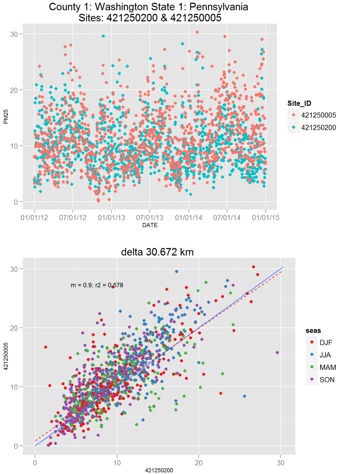
Figure 143: Comparison of PM 2.5 data for sites 421250200 and 421250005. Top panel shows time series for both sites for years 2012-2014. Bottom panel shows scatter plot of paired data, along with slope for the linear regression and correlation coefficient (r 2 ), with data points are colored by month.
