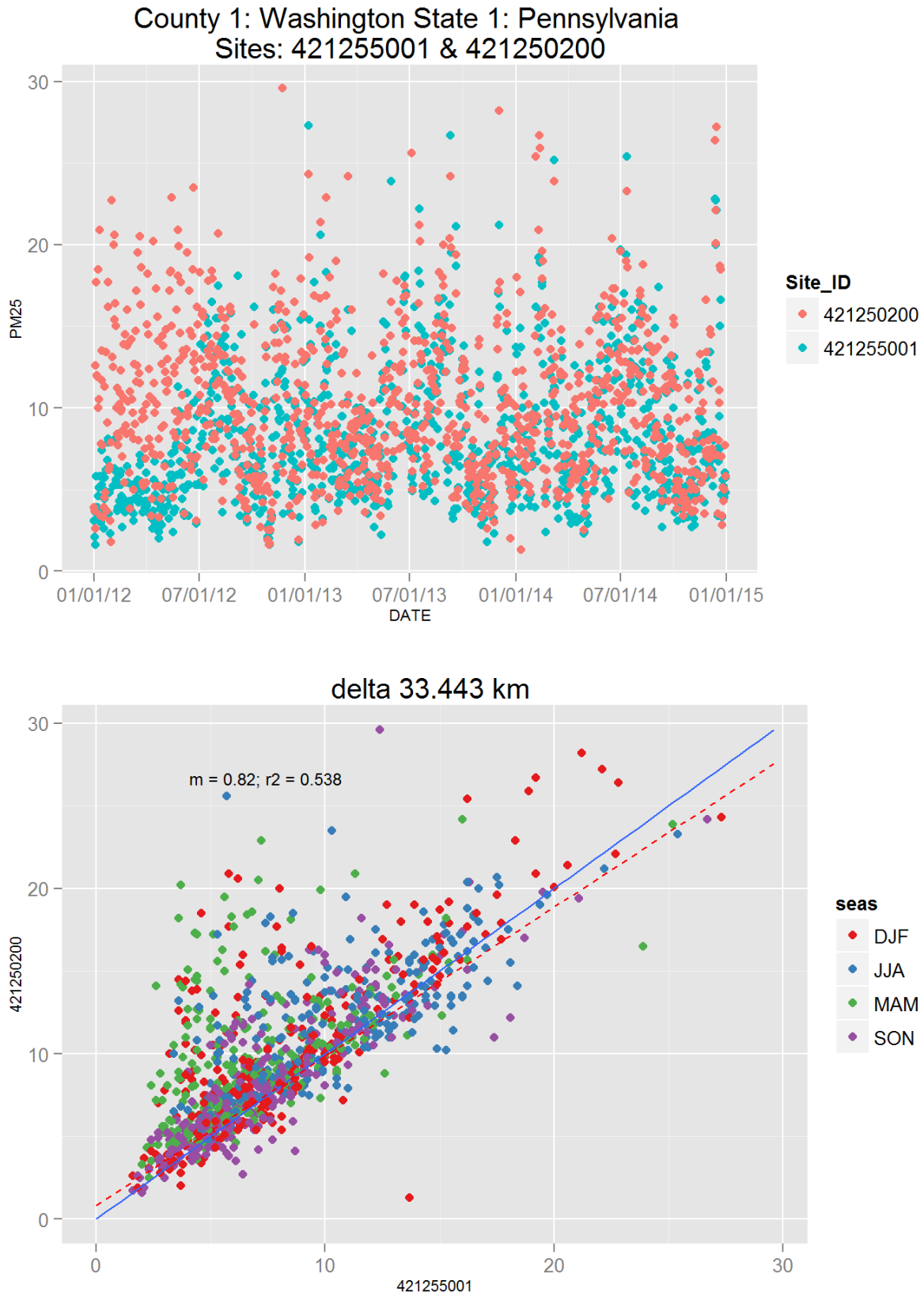
Figure 144: Comparison of PM 2.5 data for sites 421255001 and 421250200. Top panel shows time series for both sites for years 2012-2014. Bottom panel shows scatter plot of paired data, along with slope for the linear regression and correlation coefficient (r 2 ), with data points are colored by month.
