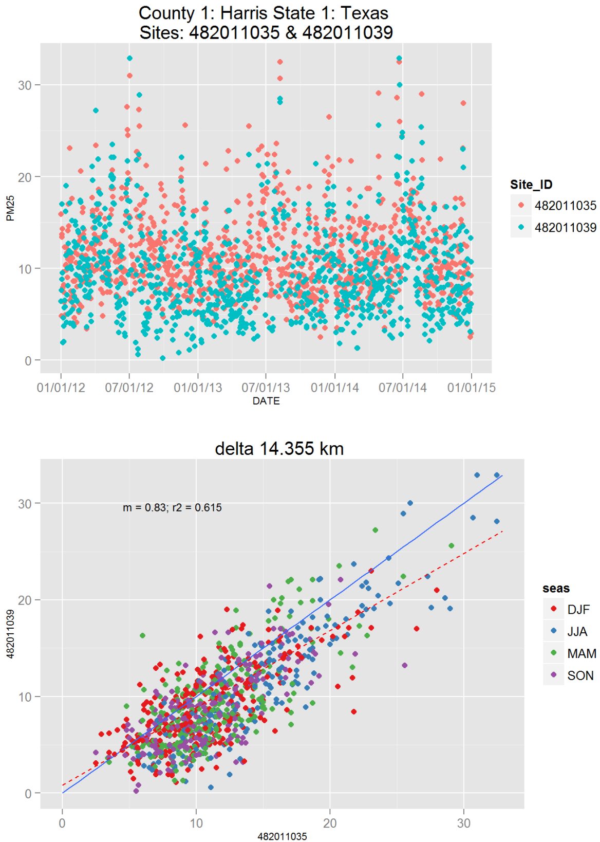
Figure 152: Comparison of PM 2.5 data for sites 482011035 and 482011039. Top panel shows time series for both sites for years 2012-2014. Bottom panel shows scatter plot of paired data, along with slope for the linear regression and correlation coefficient (r 2 ), with data points are colored by month.
