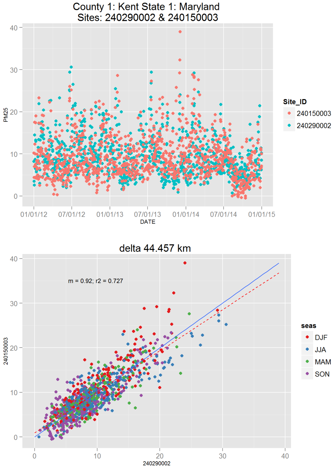
Figure 108: Comparison of PM 2.5 data for sites 240290002 and 240290002. Top panel shows time series for both sites for years 2012-2014. Bottom panel shows scatter plot of paired data, along with slope for the linear regression and correlation coefficient (r 2 ), with data points are colored by month.
