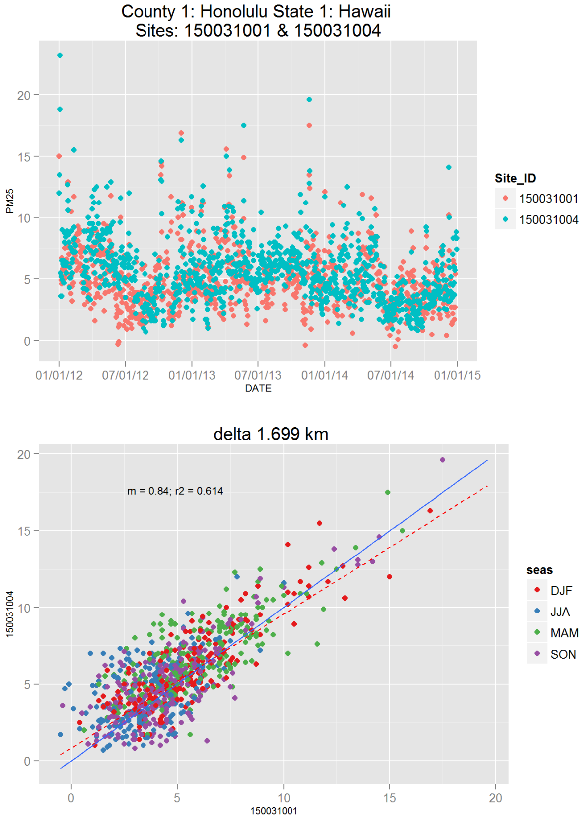
Figure 97: Comparison of PM 2.5 data for sites 150031001 and 150031004. Top panel shows time series for both sites for years 2012-2014. Bottom panel shows scatter plot of paired data, along with slope for the linear regression and correlation coefficient (r 2 ), with data points are colored by month.
