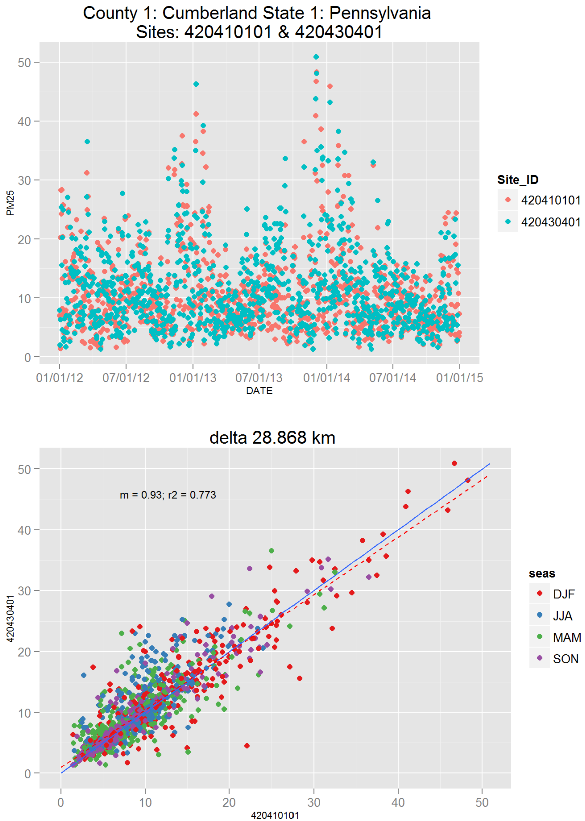
Figure 135: Comparison of PM 2.5 data for sites 420410101 and 420410101. Top panel shows time series for both sites for years 2012-2014. Bottom panel shows scatter plot of paired data, along with slope for the linear regression and correlation coefficient (r2), with data points are colored by month.
