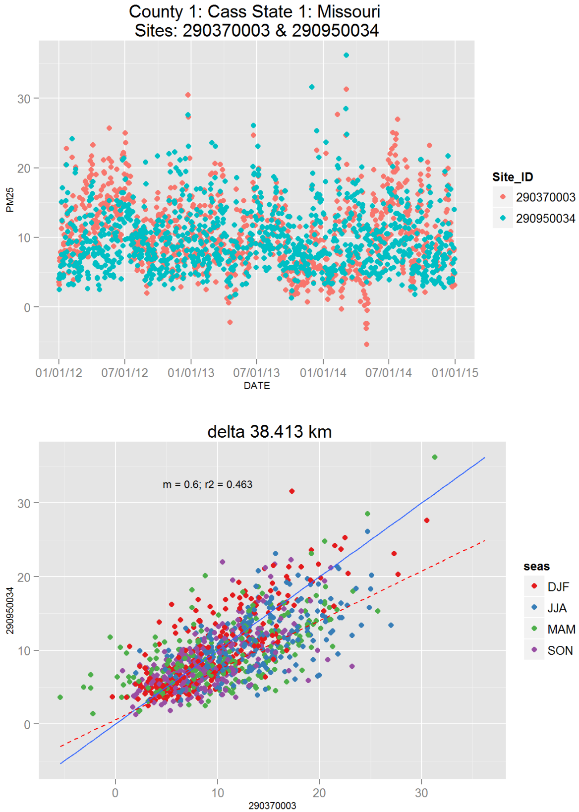
Figure 115: Comparison of PM 2.5 data for sites 290370003 and 290370003. Top panel shows time series for both sites for years 2012-2014. Bottom panel shows scatter plot of paired data, along with slope for the linear regression and correlation coefficient (r2), with data points are colored by month.
