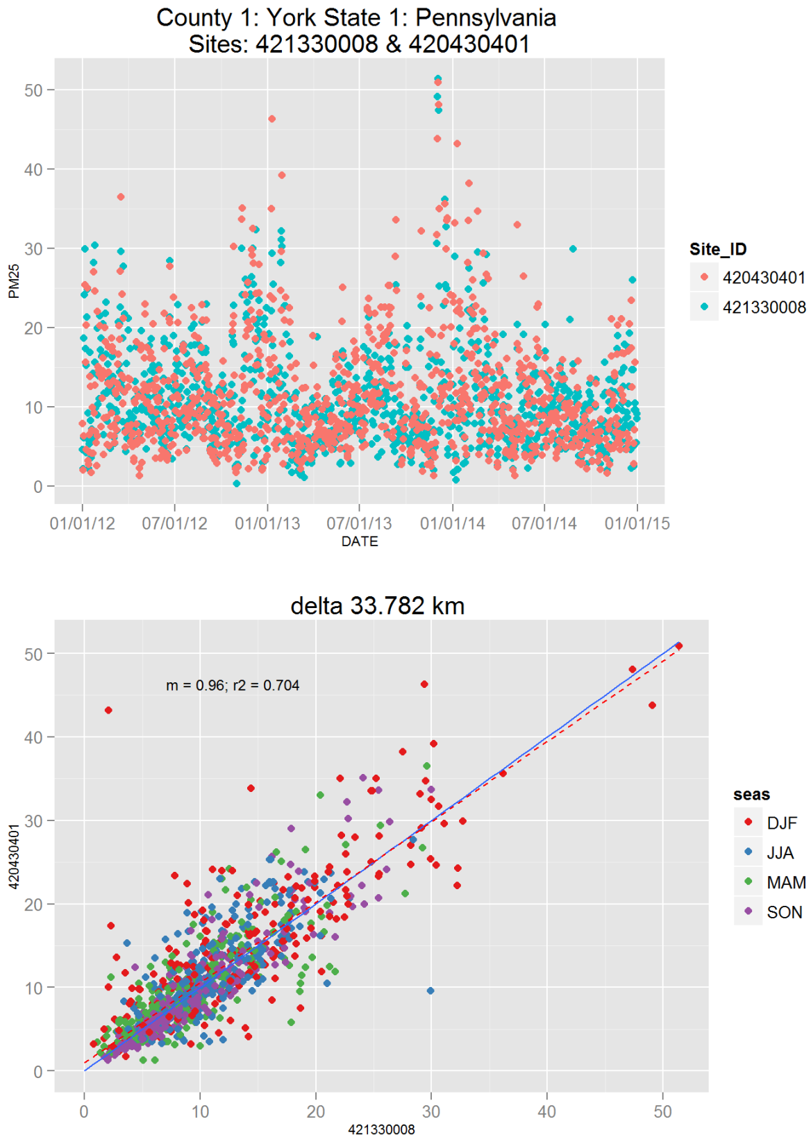
Figure 146: Comparison of PM 2.5 data for sites 421330008 and 421330008. Top panel shows time series for both sites for years 2012-2014. Bottom panel shows scatter plot of paired data, along with slope for the linear regression and correlation coefficient (r 2 ), with data points are colored by month.
