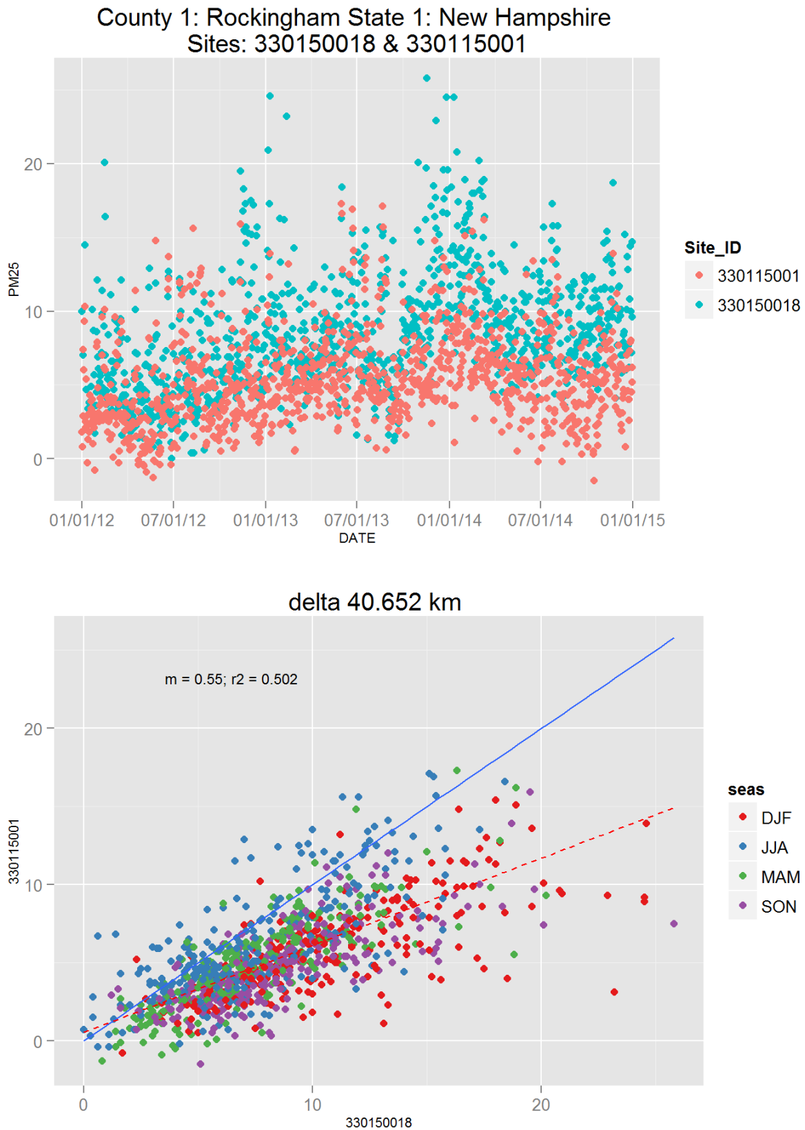
Figure 125: Comparison of PM 2.5 data for sites 330150018 and 330115001. Top panel shows time series for both sites for years 2012-2014. Bottom panel shows scatter plot of paired data, along with slope for the linear regression and correlation coefficient ( r^2 ), with data points are colored by month.
