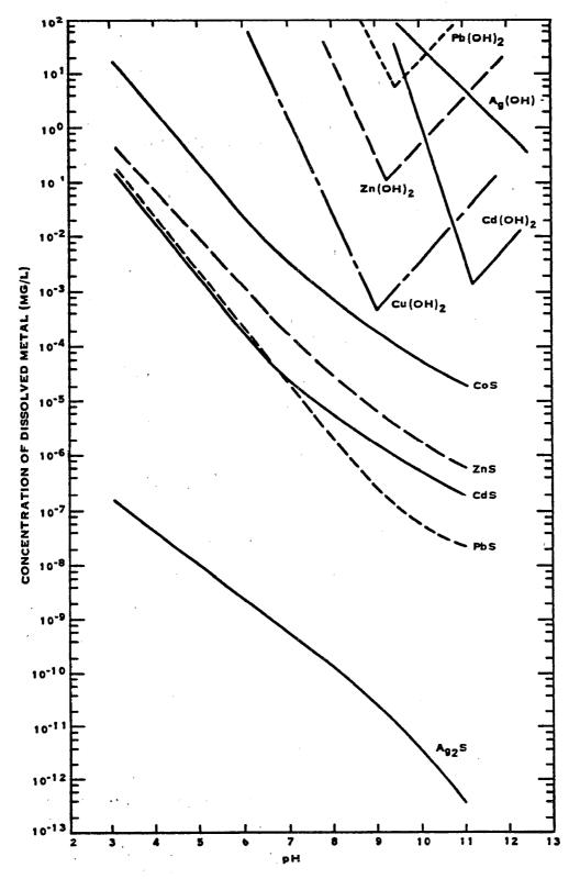
FIGURE VII-1. COMPARATIVE SOLUBILITIES OF METAL HYDROXIDES AND SULFIDE AS A FUNCTION OF pH
