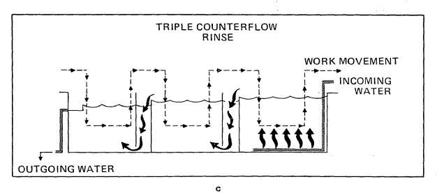
Figure VII-37 COUNTER CURRENT RINSING (TANKS)
