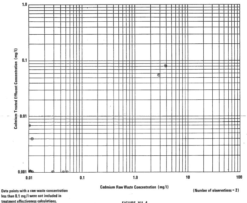
FIGURE VII-4 HYDROXIDE PRECIPITATION SEDIMENTATION EFFECTIVENESS CADMIUM
