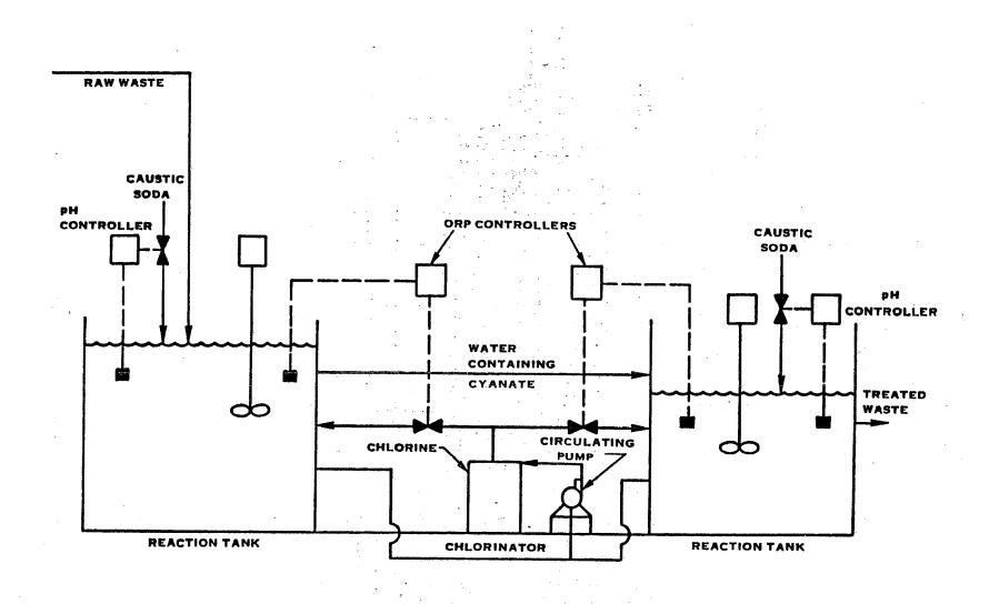
FIGURE VII-19. TREATMENT OF CYANIDE WASTE BY ALKALINE CHLORINATION
