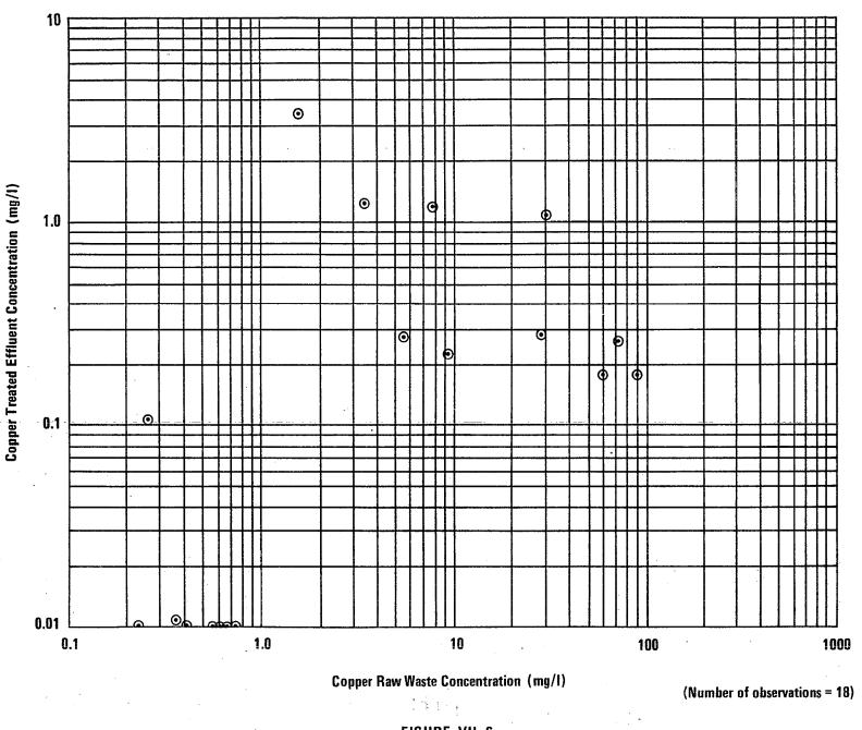
FIGURE VII-6 HYDROXIDE PRECIPITATION SEDIMENTATION EFFECTIVENESS COPPER
