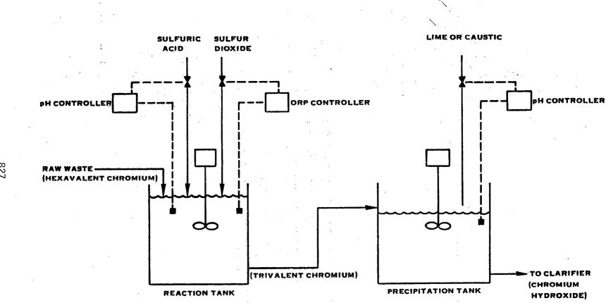
FIGURE VII-13. HEXAVALENT CHROMIUM REDUCTION WITH SULFUR DIOXIDE
