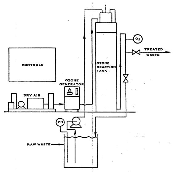
FIGURE VII-20. TYPICAL OZONE PLANT FOR WASTE TREATMENT
