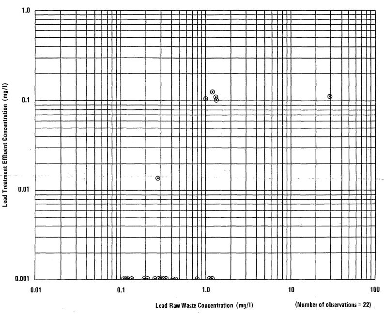
FIGURE VII-7 HYDROXIDE PRECIPITATION SEDIMENTATION EFFECTIVENESS
