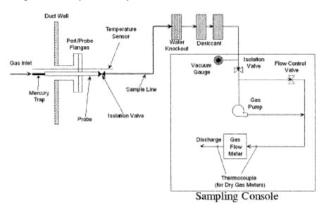
Figure 12B-1. Typical Sorbent Trap Monitoring System (only one trap and associated sampling system is illustrated).
