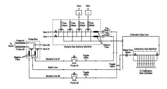
Figure 1. Extractive FTIR sampling system.
