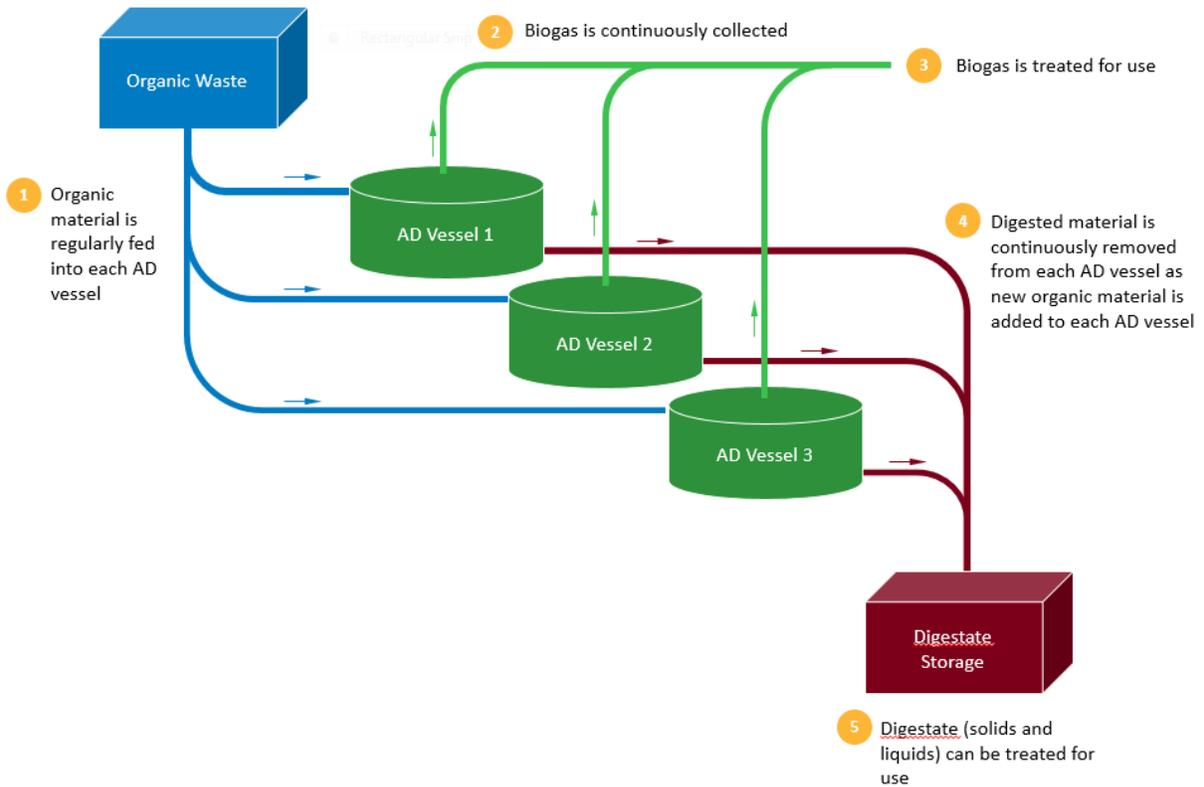
**Phased Continuous Flow System with a Series of Vessels**
