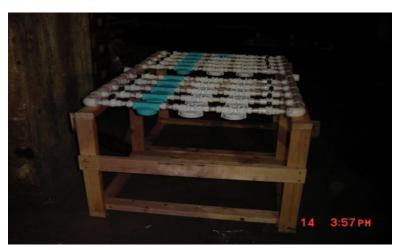
Figure 6. A filter array that is designed to hold filters of sequentially decreasing pore size.
