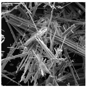
Figure 1. The fibrous mineral anthophyllite asbestos as seen using TEM.
