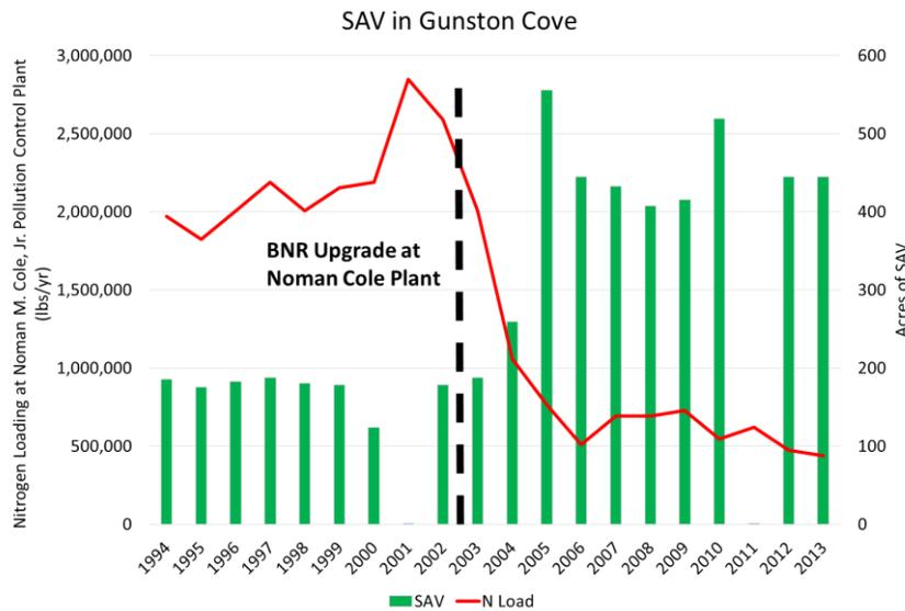
Wastewater treatment plant upgrades to BNR in the metropolitan Washington, D.C. area resulted in reductions in phosphorus and nitrogen concentrations. These nutrient reductions led to decreases in toxic cyanobacteria and helped submerged aquatic vegetation recover in the tidal Potomac River, such as those shown at Gunston Cove in Fairfax, Virginia. Note: 2001 and 2011 data not available. ([bit.ly/ChesBayInsights](http://bit.ly/ChesBayInsights))
