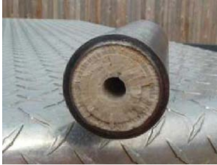
Figure D-19. Barium Sulfate Scaling in Haynesville Shale Pipe
