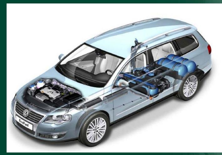
Dual Fuel CNG / Gasoline VW Passat
