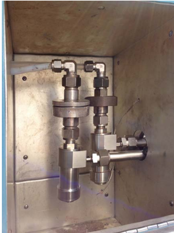
Figure 3-5. Dual PM 2.5 Cyclone/Filter Assemblies in Dual Train Hot Box
