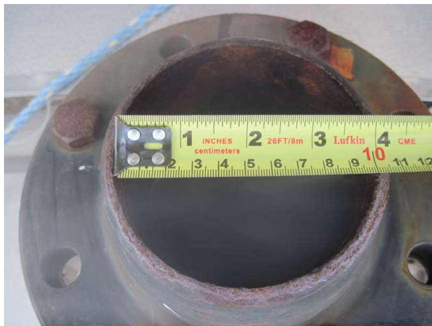
Figure 3-1. Sampling Port Internal Diameter
