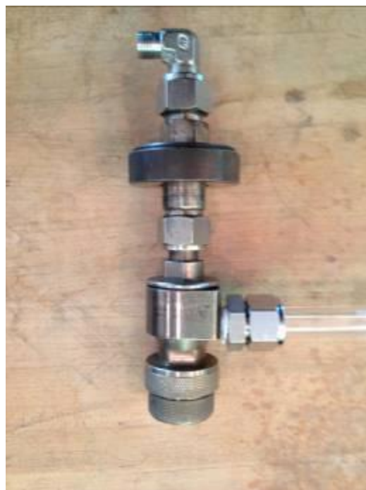
Figure 2. PM 2.5 Cyclone Sampling Head and 47 mm Filter Holder (Note: standard connection to PM 2.5 cyclone is a 5/8" O.D. glass probe liner)
