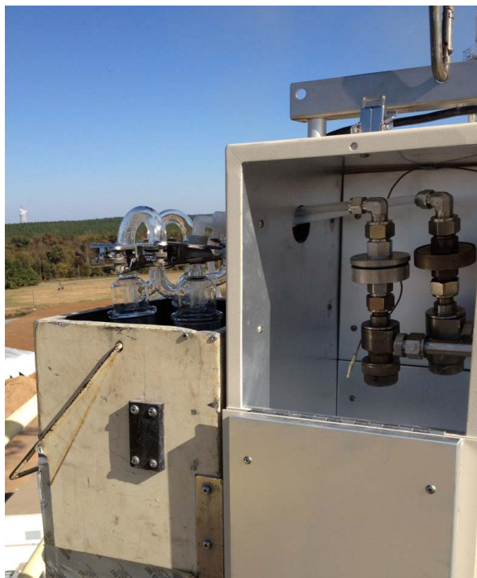
Figure 3-4. Dual Sampling Train During Method 301 Validation Tests
