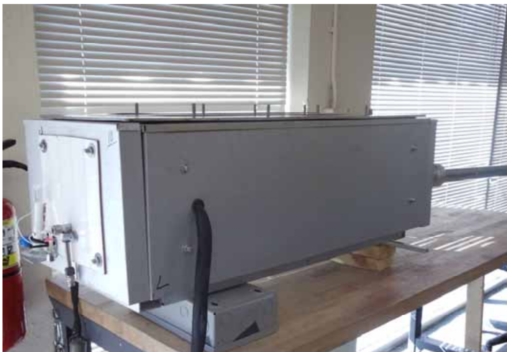
Figure 3-15. Heated Chamber and WS2.5 Sampling System Nozzle and Probe
