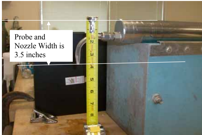
Figure 2-3. WS2.5 Heated Probe and 90 Degree Curved Nozzle
