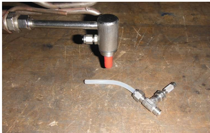
Figure 2. Precutter Nozzle with Cap Prior to the Attachment of the Needle Valve
