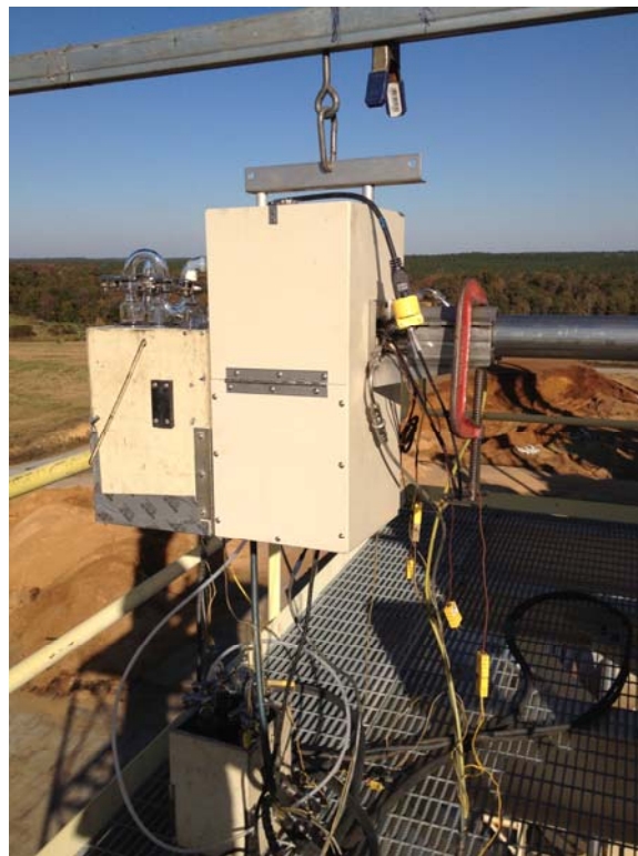
Figure 3-3. Dual Sampling Train with Two Sets of Method 4 Impingers
