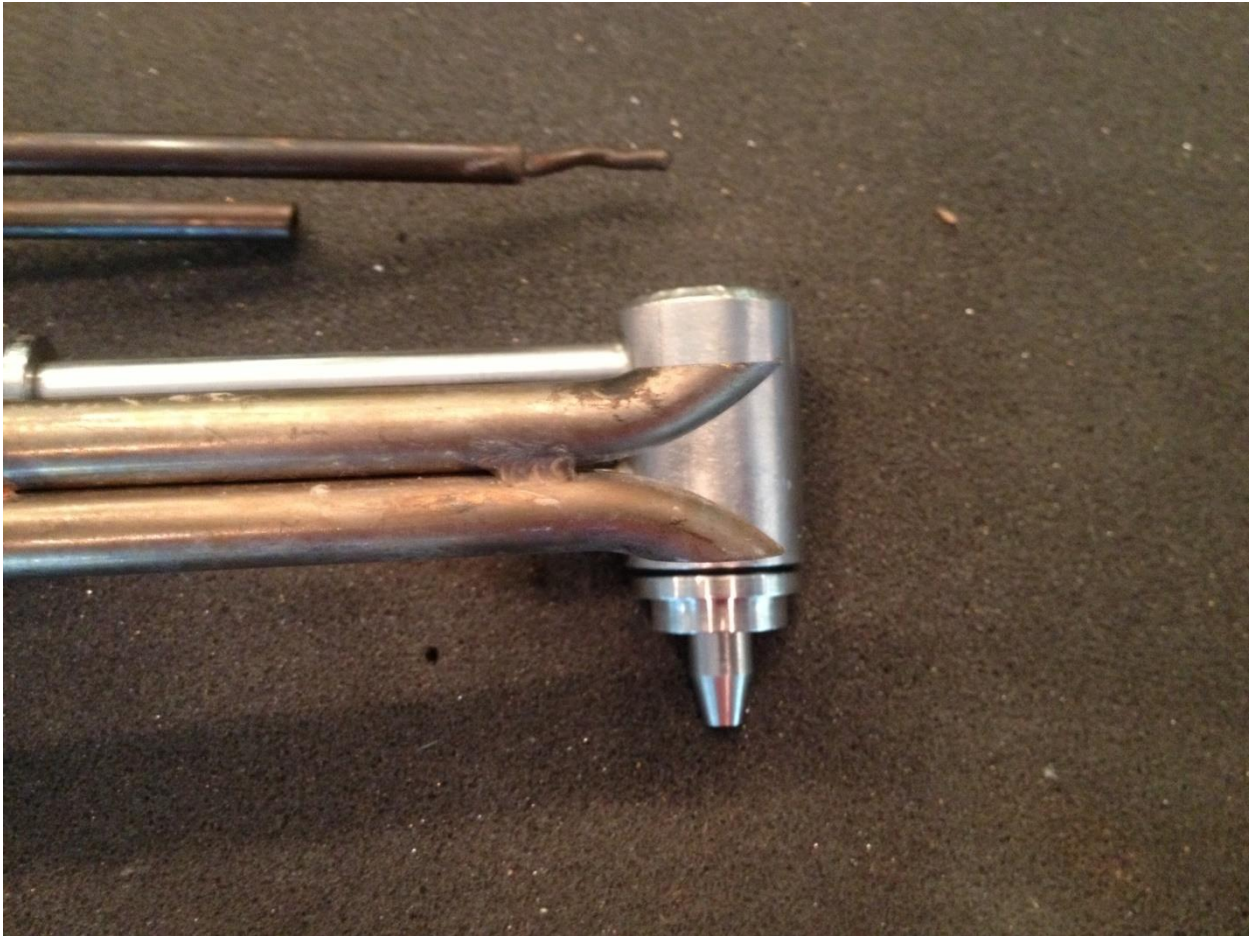
Figure 4. Precutter Nozzle Attached to Method 5 Sampling Probe
