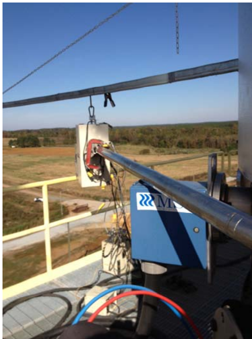
Figure 3-6. Dual Sampling Train with Two Method 4 Trains
