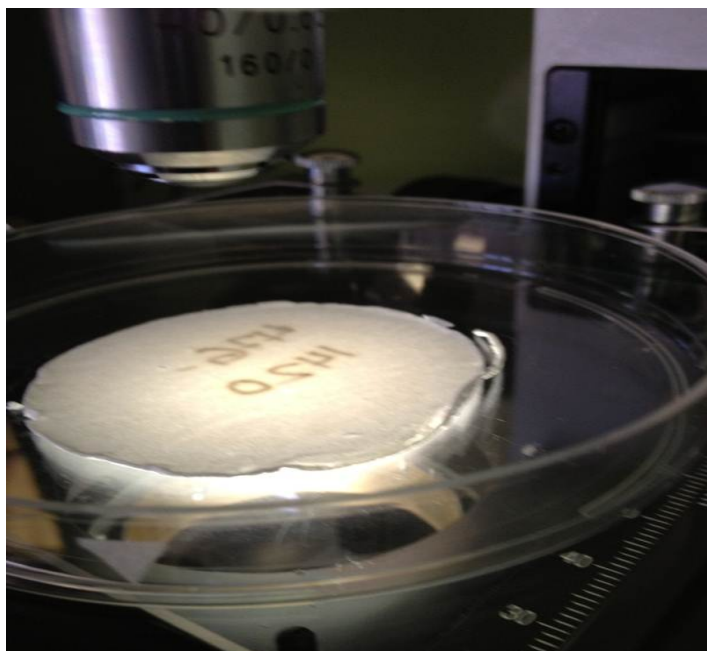
Figure 3-7. Crack in Filter S2-5
