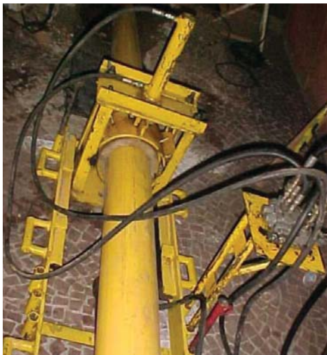
Auxiliary equipment used to insert polyethylene pipe
