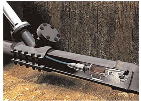
*CISBOT Enters the Gas Main Via Its Launch Tube Attached to the Bidirection Fitting. Photo Courtesy of ULC Robotics.*
