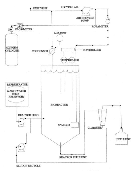
EPA METHOD 304A VENT BIOREACTOR SYSTEM
