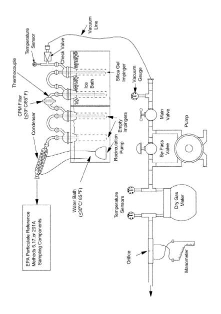
Figure 1. Schematic of Condensable Particulate Sampling Train
