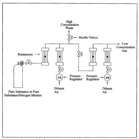
Figure 18-6. Two-Stage Dilution Apparatus.
