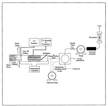
Figure 18-12. Direct Interface Sampling System.
