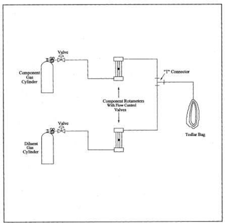
Figure 18-5. Single-Stage Calibration Gas Dilution System.
