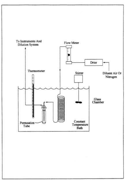
Figure 15-3. Apparatus for Field Calibration.
