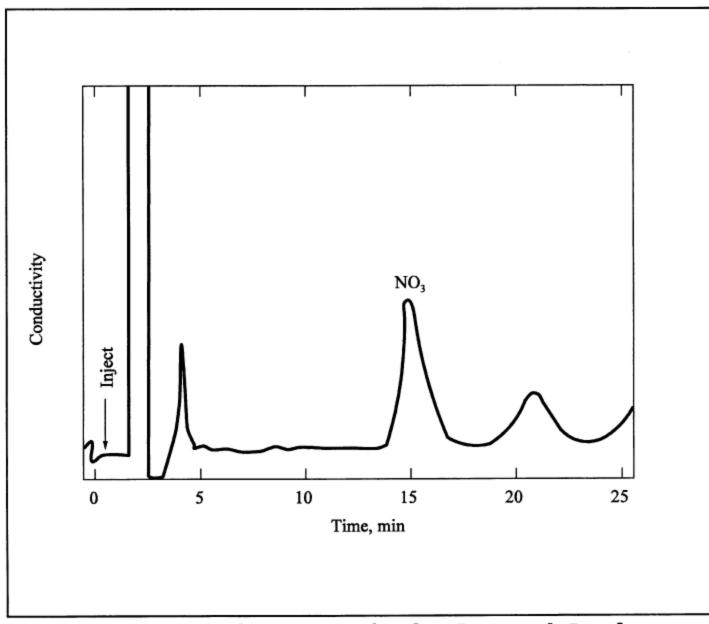
Figure 7D-1. Ion Chromatograph of a Prepared Sample.
