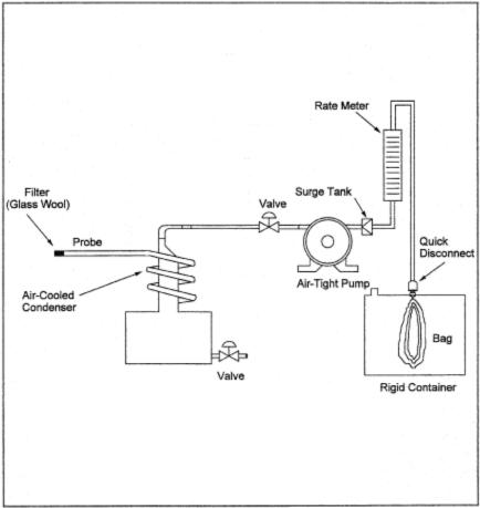
Figure 3-2. Integrated Gas-Sampling Train.
