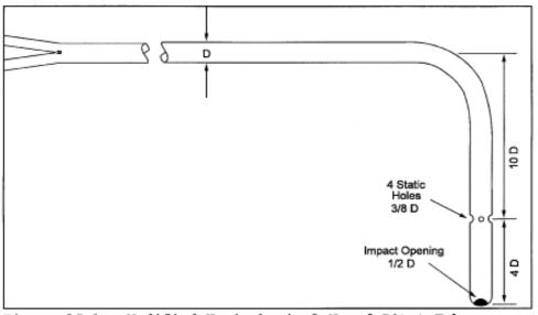
Figure 2C-1. Modified Hemispherical-Nosed Pitot Tube.
