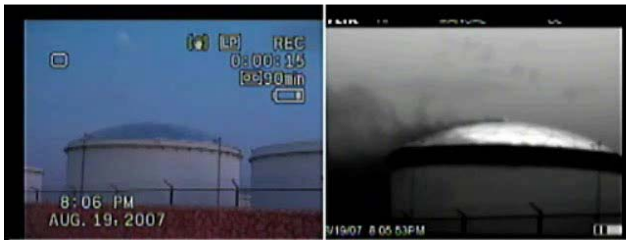
Figure 2-22. Detection of Gaseous VOC Emissions from a Chemical Storage Tank 14
