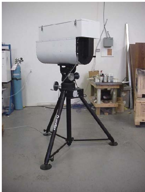
Figur2-6. Typical Telescopic FTIR Transmitting and Detection Unit
