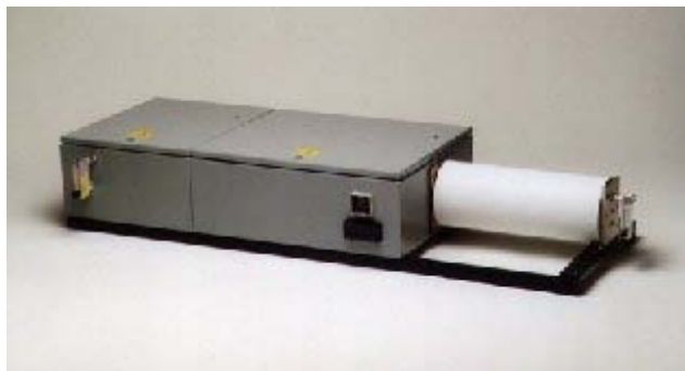
Figure 2-3. FTIR Closed Cell Unit Used to Monitor Stack Gas
