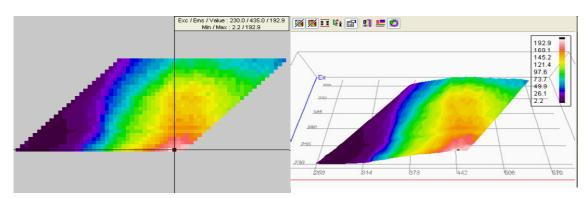
Simulation of oil contamination in water – front face measuring geometry. Drop of crude oil dissolved in water and then measured with Instant Screener Compact: 2-D SFS (left) and 3-D SFS (right) indicate the characteristic spectral pattern of oil emulsion in water (marked with red circles).
