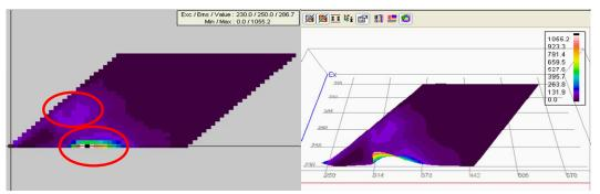
3. Simulation of contamination in water – volume measuring geometry - measured with Fluo-Imager. Development in time: maximal fluorescence intensity of oil in water was initially 319 (left SFS below), and increased up to 1457 (right SFS below) in 24 hours due to extraction of aromatic compounds in water.
