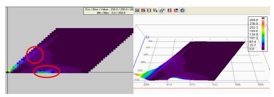
The same sample measured again with Instant Screener Compact after 24 h: the spectral pattern of oil remains the same while the fluorescence intensity increased 5 times due to extraction of oil into water with time.
